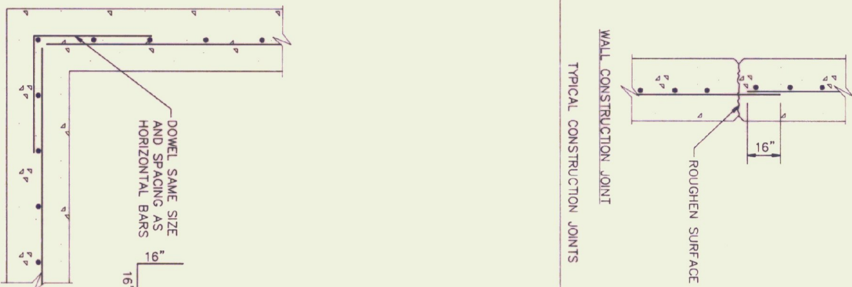
DETAIL TYPICAL CORNER REINFORCING SCALE: NONE 20
