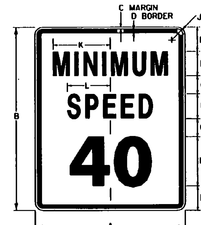
• OPTICALLY SPACE NUMERALS ABOUT VERTICAL CENTERLINE. R2-4
