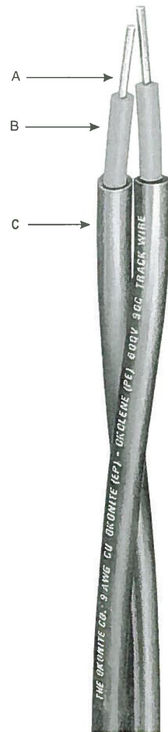
A Bare Copper Conductor- Size #9 AWG, #6 AWG Solid B Insulation - Okonite-Sizes #9 AWG and #8 AWG-5/64", #6 AWG-6/64" C Jacket-Okolene, Color Coded; 1-Black, 1-Red
