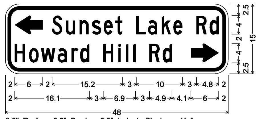
3.0" Radius, 0.8" Border, 0.5" Indent, Black on Yellow; Standard Arrow Custom 6.0" X 4.0" 180°; [Sunset Lake Rd] C 78% spacing; [Howard Hill Rd] C 80% spacing; Standard Arrow Custom 6.0" X 4.0" 0°; W16-8aP
