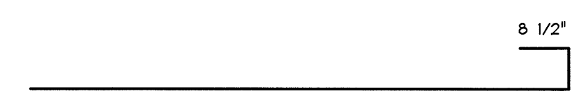
CA-601D #6 BENT BAR LEVEL II (DUAL COATED) USE 3 3/4" \phi (95 mm) PIN (60) REQ'D.
