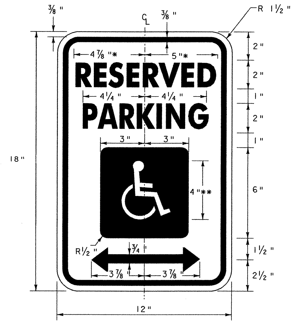
R7-8 GREEN LEGEND & BORDER WHITE SYMBOL ON BLUE BACKGROUND WHITE (REFL.) BACKGROUND SEE VTrans STANDARD E-143 FOR MATERIALS
