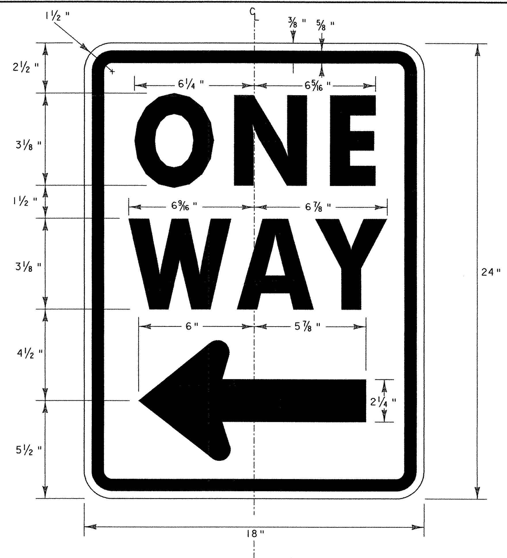
BLACK BORDER, TEXT & SYMBOL WITH WHITE REFLECTORIZED BACKGROUND SEE VTrans STANDARD E-142 FOR MATERIALS LOCATIONS STA. 0+25, RT.
