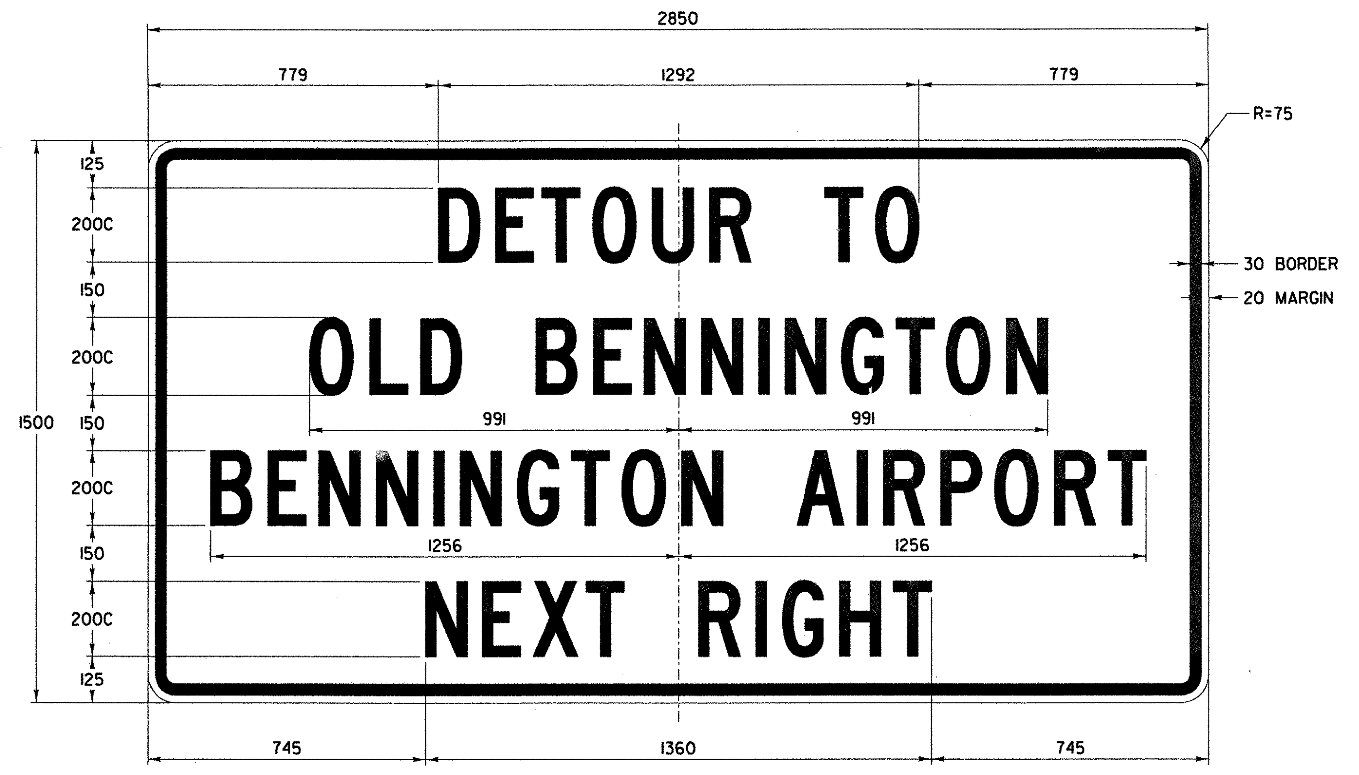
COLOR: BLACK BORDER & TEXT (REFLECTORIZED) ORANGE BACKGROUND (REFLECTORIZED)
