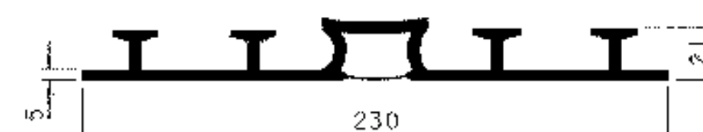
P.V.C. WATERSTOP FOR EXPANSION JOINTS NOT TO SCALE
