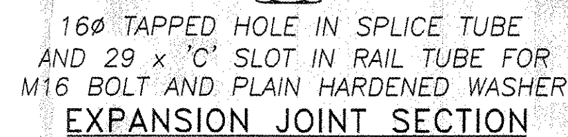
EXPANSION JOINT SECTION
