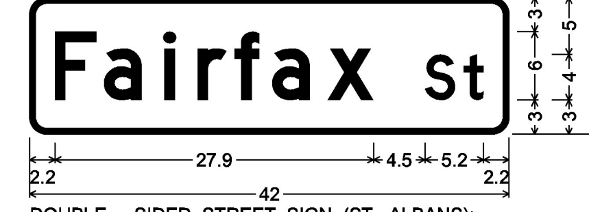
DOUBLE - SIDED STREET SIGN (ST. ALBANS); 1.5" Radius, 0.5" Border, White on Green; [Fairfax St] D;
