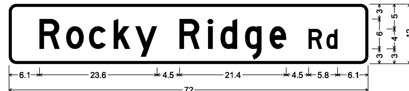
DOUBLE - SIDED STREET SIGN (FAIRFAX); 1.5" Radius, 0.5" Border, White on Green; [Rocky Ridge Rd] D;
