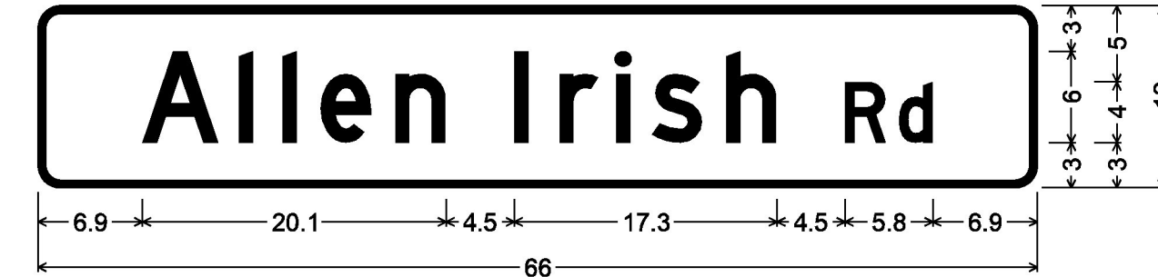
DOUBLE - SIDED STREET SIGN (FAIRFAX); 1.5" Radius, 0.5" Border, White on Green; [Allen Irish Rd] D;
