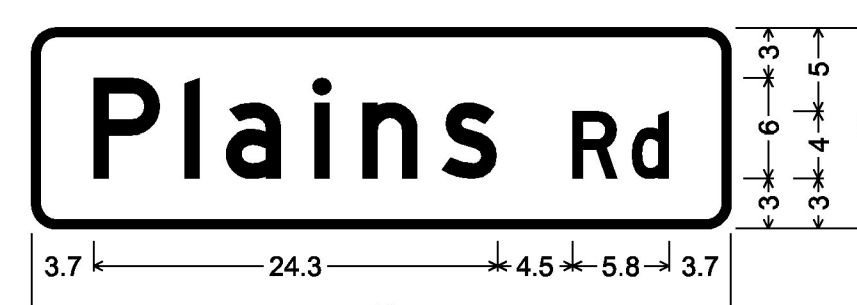
DOUBLE - SIDED STREET SIGN (FAIRFAX); 1.5" Radius, 0.5" Border, White on Green; [Plains Rd] D;
