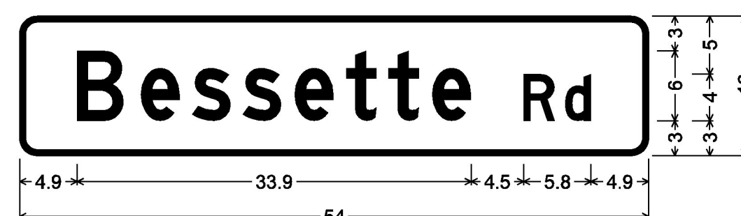
DOUBLE - SIDED STREET SIGN (FAIRFAX); 1.5" Radius, 0.5" Border, White on Green; [Bessette Rd] D;
