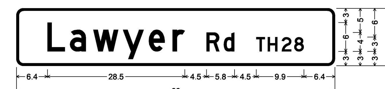
DOUBLE - SIDED STREET SIGN (BAKERSFIELD); 1.5" Radius, 0.5" Border, White on Green; [Lawyer Rd TH28] D;
