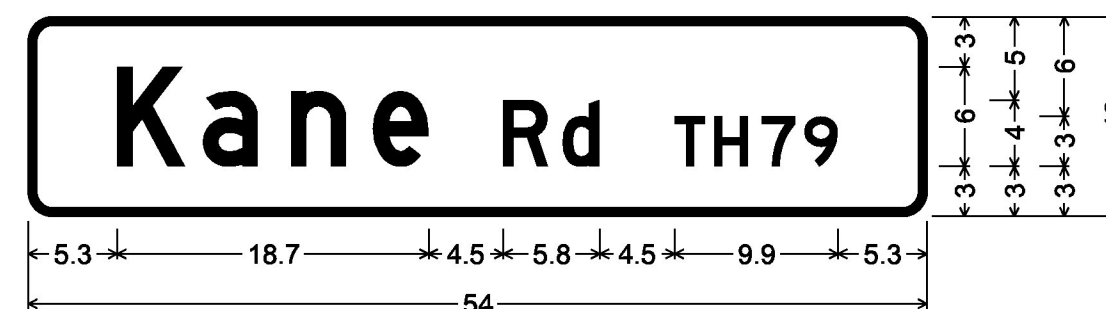
DOUBLE - SIDED STREET SIGN (FAIRFIELD); 1.5" Radius, 0.5" Border, White on Green; [Kane Rd TH79] D;
