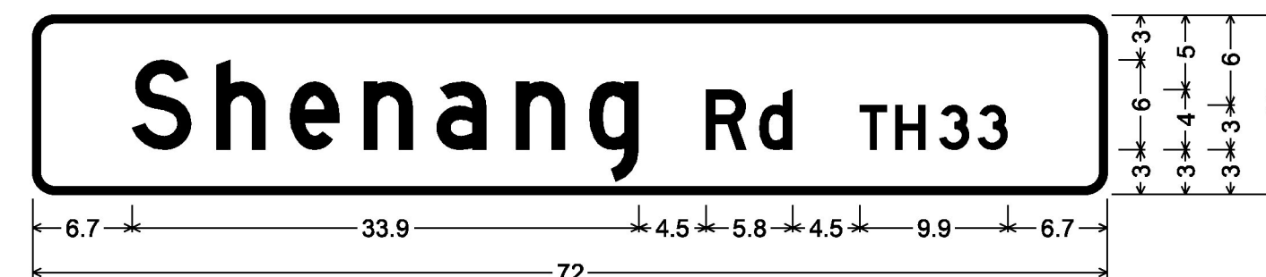
DOUBLE - SIDED STREET SIGN (FAIRFIELD); 1.5" Radius, 0.5" Border, White on Green; [Shenang Rd TH33] D;
