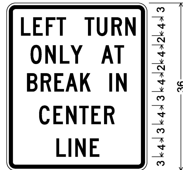
W16-18P; 1.500" Radius, 0.625" Border, 0.375" Indent, Black on Fluorescent Yellow; [NOTICE] D 2K specified length;
