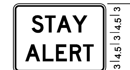
1.500" Radius, 0.375" Border, 0.375" Indent, Black on Yellow; [STAY] D 2K; [ALERT] D 2K;
