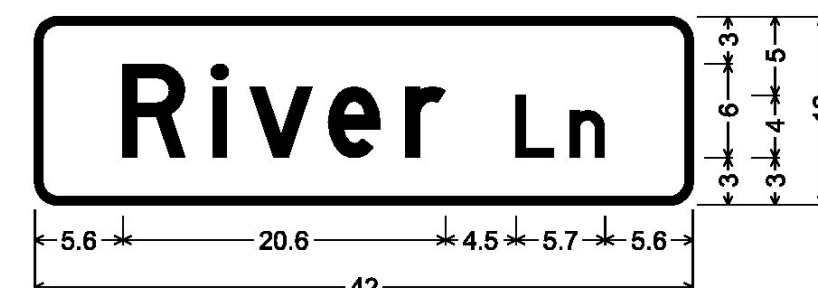
DOUBLE-SIDED STREET SIGN (NEWARK); 1.5" Radius, 0.5" Border, White on Green; [River Ln] D;
