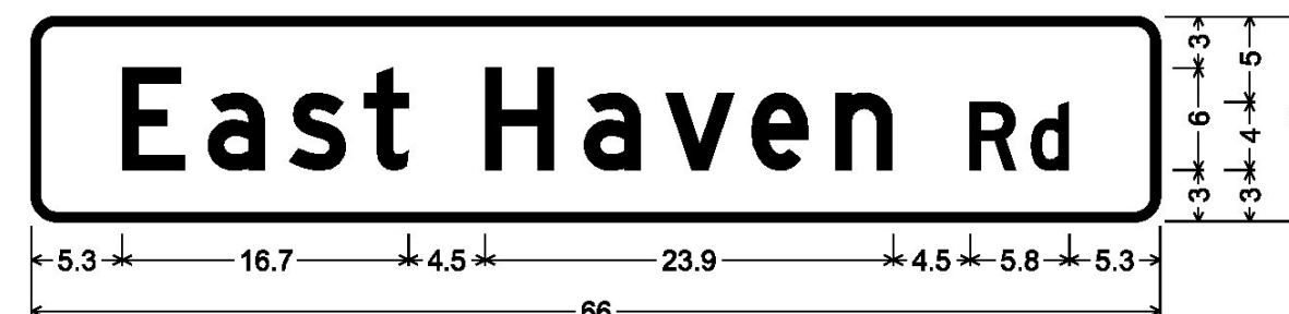
DOUBLE-SIDED STREET SIGN (BRIGHTON); 1.5" Radius, 0.5" Border, White on Green; [East] D [ ] C [Haven Rd] D;
