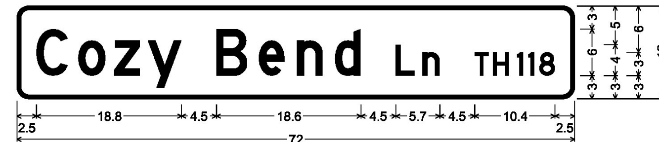
DOUBLE-SIDED STREET SIGN (LYNDON); 1.5" Radius, 0.5" Border, White on Green; [Cozy] D [ ] C [Bend Ln TH118] D;
