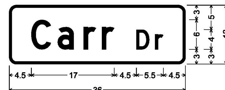
DOUBLE-SIDED STREET SIGN (BURKE); 1.5" Radius, 0.5" Border, White on Green; [Carr Dr] D;
