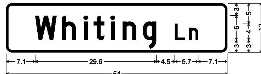
DOUBLE-SIDED STREET SIGN (BROWNINGTON); 1.5" Radius, 0.5" Border, White on Green; [Whiting Ln] D;
