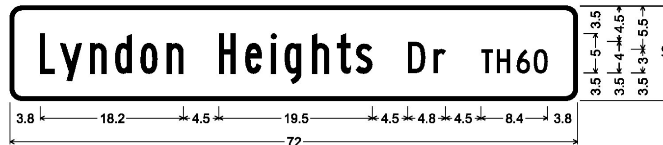
DOUBLE - SIDED STREET SIGN (LYNDON); 1.5" Radius, 0.5" Border, White on Green; [Lyndon] B [ ] D [Heights] B [ ] D [Dr TH60] C;
