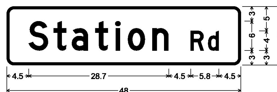
DOUBLE-SIDED STREET SIGN (SUTTON); 1.5" Radius, 0.5" Border, White on Green; [Station Rd] D;
