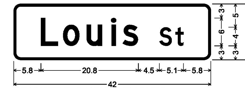
DOUBLE-SIDED STREET SIGN (DERBY); 1.5" Radius, 0.5" Border, White on Green; [Louis St] D;
