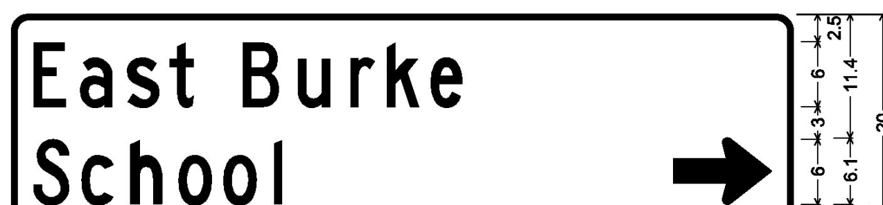
1.5" Radius, 0.5" Border, White on Green; [East Burke] C; [School] C; Standard Arrow Custom 9.0" X 6.1" 0°;
