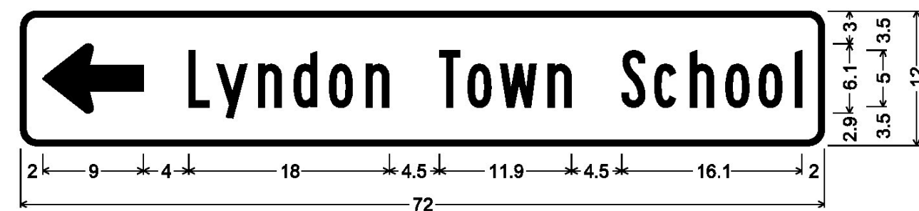
1.5" Radius, 0.5" Border, White on Green; Standard Arrow Custom 9.0" X 6.1" 180°; [Lyndon] Town School] B 96% spacing;
