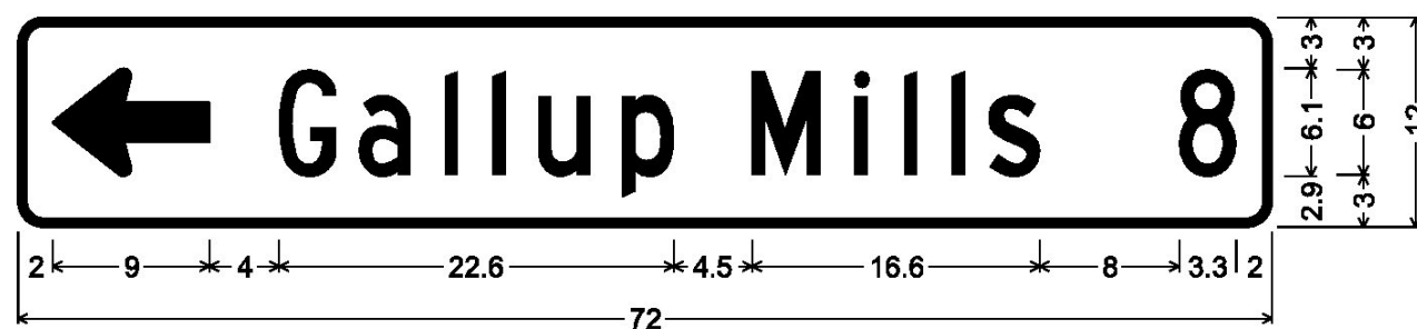
1.5" Radius, 0.5" Border, White on Green; Standard Arrow Custom 9.0" X 6.1" 180°; [Gallup Mills 8] C;
