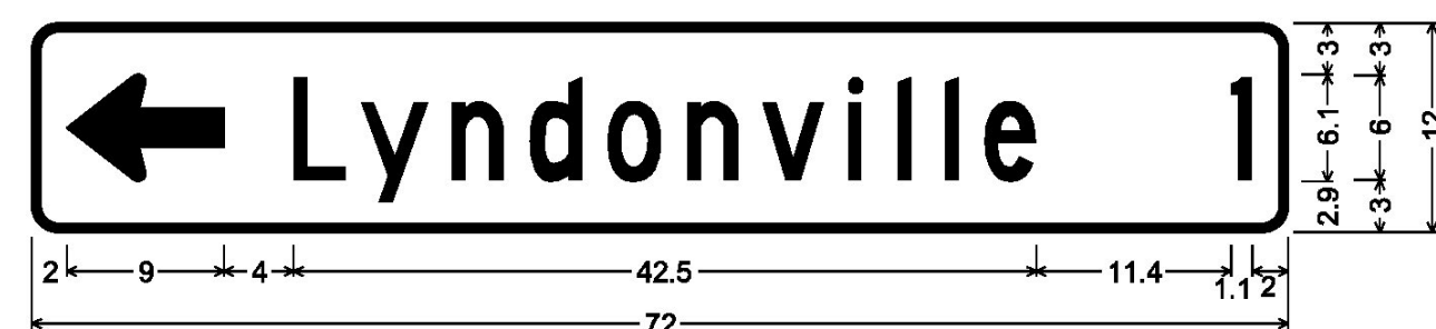
1.5" Radius, 0.5" Border, White on Green; Standard Arrow Custom 9.0" X 6.1" 180°; [Lyndonville] C; [1] C;
