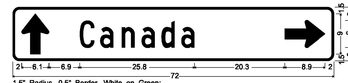
1.5" Radius, 0.5" Border, White on Green; Standard Arrow Custom 9.0" X 6.1" 90°; [Canada] C; Standard Arrow Custom 9.0" X 6.1" 0°;
