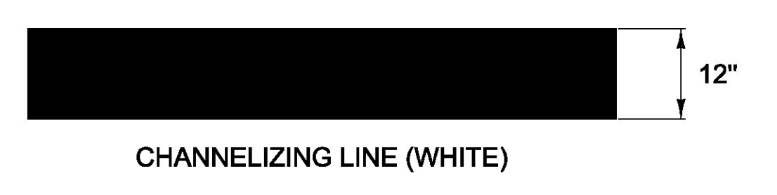
PAVEMENT MARKING LINE DETAILS
