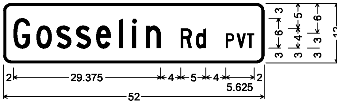
Double-Sided Street Sign (Calais); 1.500" Radius, 0.500" Border, White on Green; [Gosselin] C; [Rd] C; [PVT] C;
