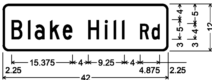
Double-Sided Street Sign (Woodbury); 1.500" Radius, 0.500" Border, White on Green; [Blake Hill] C 90% spacing; [Rd] C 90% spacing;
