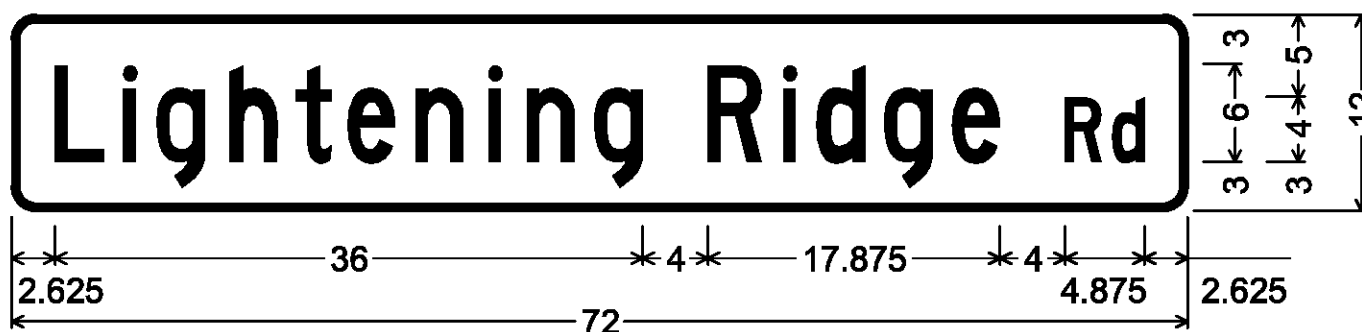
Double-Sided Street Sign (Calais); 1.500" Radius, 0.500" Border, White on Green; [Lightening Ridge] C 80% spacing; [Rd] C 80% spacing;
