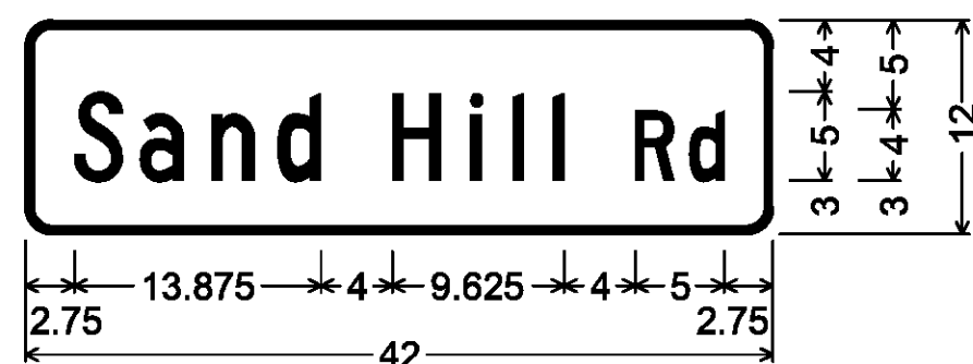
Double-Sided Street Sign (Calais); 1.500" Radius, 0.500" Border, White on Green; [Sand Hill] C; [Rd] C;
