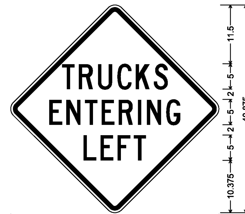
30.000" across sides 1.875" Radius, 0.750" Border, 0.500" Indent, Black on Yellow; [TRUCKS] C; [ENTERING] C; [LEFT] C;
