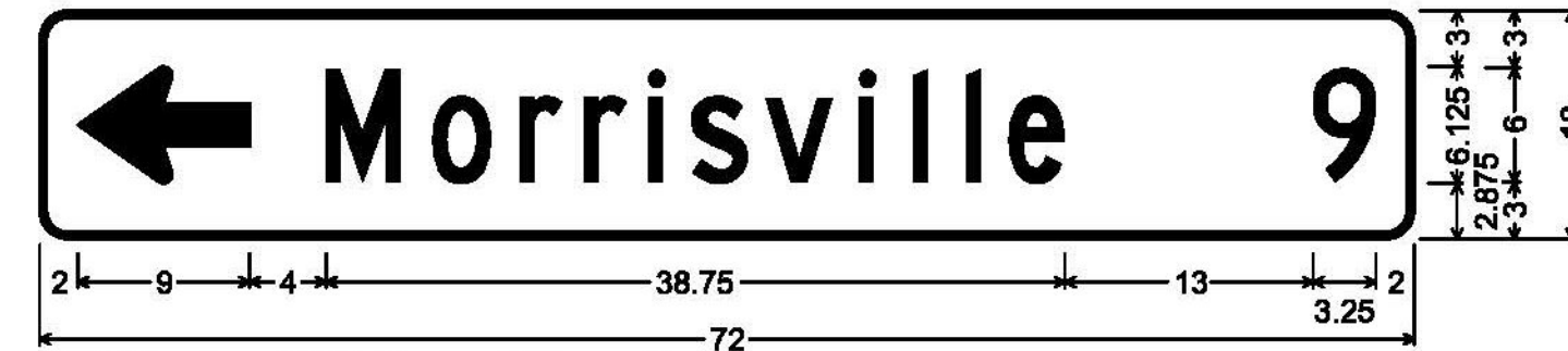
1.500" Radius, 0.375" Border, White on Green; Standard Arrow Custom 9.000" X 6.125" 180"; [Morrisville] C; [9] C;
