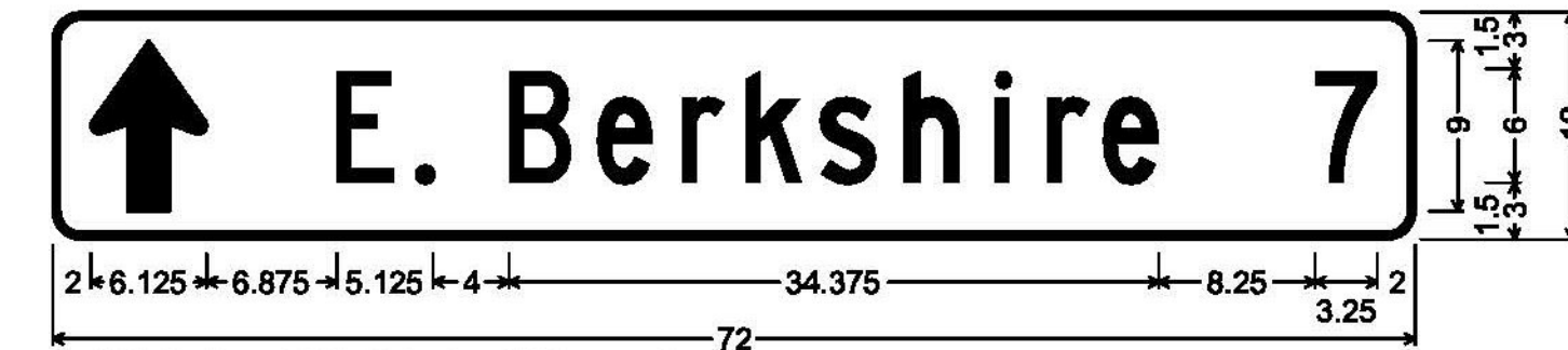
1.500" Radius, 0.375" Border, White on Green; Standard Arrow Custom 9.000" X 6.125" 90"; [E. Berkshire] C; [7] C;
