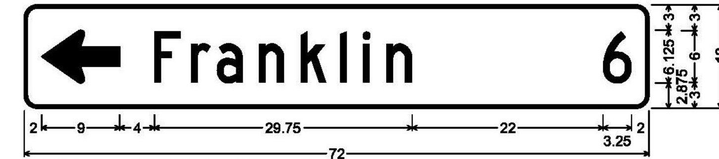
1.500" Radius, 0.375" Border, White on Green; Standard Arrow Custom 9.000" X 6.125" 180"; [Franklin] C; [6] C;
