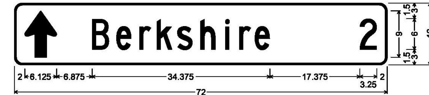
1.500" Radius, 0.375" Border, White on Green; Standard Arrow Custom 9.000" X 6.125" 90"; [Berkshire] C; [2] C;
