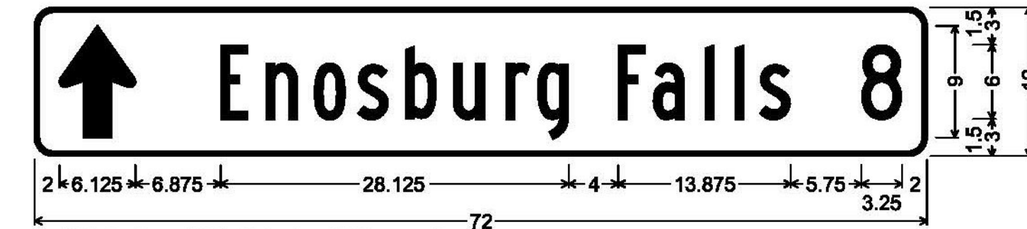
1.500" Radius, 0.375" Border, White on Green; Standard Arrow Custom 9.000" X 6.125" 90"; [Enosburg Falls] B; [8] C;
