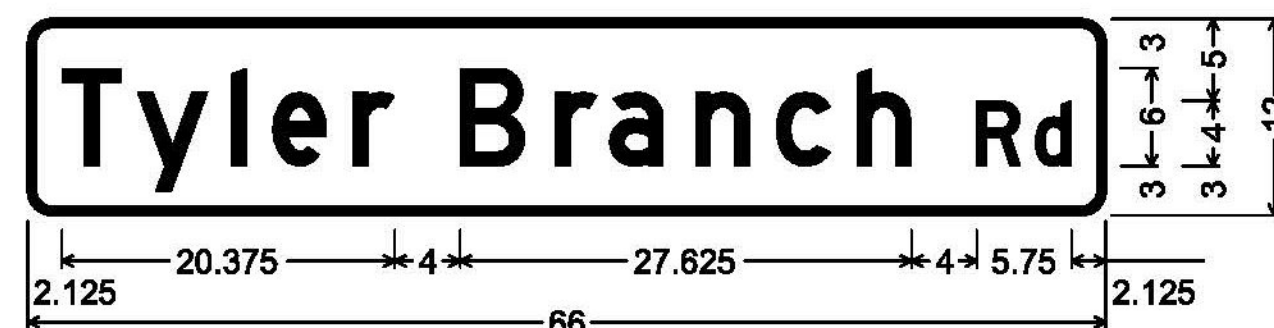
DOUBLE-SIDED STREET SIGN (ENOSBURGH); 1.500" Radius, 0.500" Border, White on Green; [Tyler Branch] D; [Rd] D;
