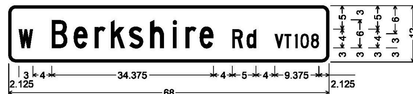
DOUBLE-SIDED STREET SIGN (BERKSHIRE); 1.500" Radius, 0.500" Border, White on Green; [W] C; [Berkshire] C; [Rd] C; [VT108] C;
