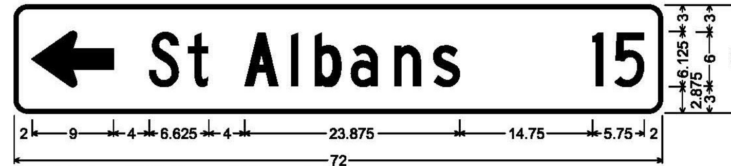
1.500" Radius, 0.375" Border, White on Green; Standard Arrow Custom 9.000" X 6.125" 180"; [St Albans] C; [15] C;
