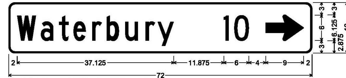
1.500" Radius, 0.375" Border, White on Green; [Waterbury] C; [10] C; Standard Arrow Custom 9.000" X 6.125" 0°;
