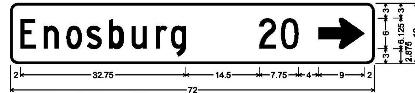
1.500" Radius, 0.375" Border, White on Green; [Enosburg] C; [20] C; Standard Arrow Custom 9.000" X 6.125" 0°;
