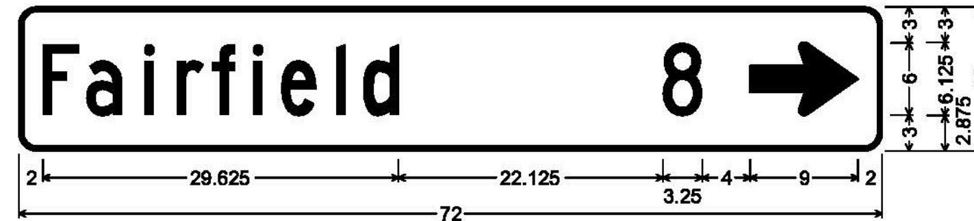
1.500" Radius, 0.375" Border, White on Green; [Fairfield] C; [8] C; Standard Arrow Custom 9.000" X 6.125" 0°;
