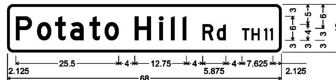
DOUBLE-SIDED STREET SIGN (BERKSHIRE); 1.500" Radius, 0.500" Border, White on Green; [Potato Hill] D; [Rd] D; [TH11] D;
