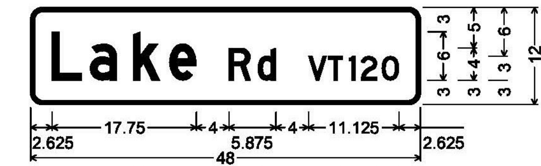
DOUBLE-SIDED STREET SIGN (BERKSHIRE); 1.500" Radius, 0.500" Border, White on Green; [Lake] D; [Rd] D; [VT120] D;
