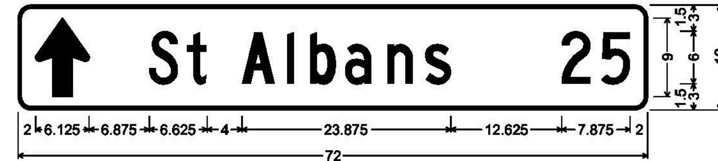
1.500" Radius, 0.375" Border, White on Green; Standard Arrow Custom 9.000" X 6.125" 90"; [St Albans] C; [25] C;
