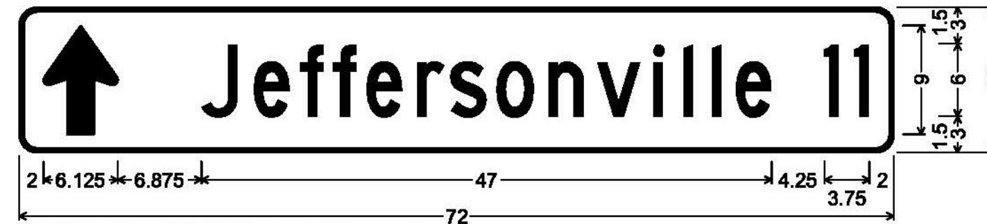
1.500" Radius, 0.375" Border, White on Green; Standard Arrow Custom 9.000" X 6.125" 90"; [Jeffersonville] C 80% spacing; [11] C;
