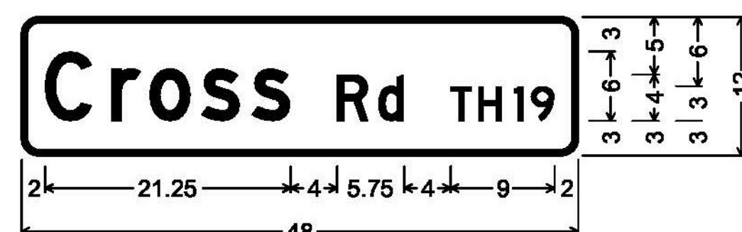
DOUBLE-SIDED STREET SIGN (BERKSHIRE); 1.500" Radius, 0.500" Border, White on Green; [Cross] D; [Rd] D; [TH19] D;
