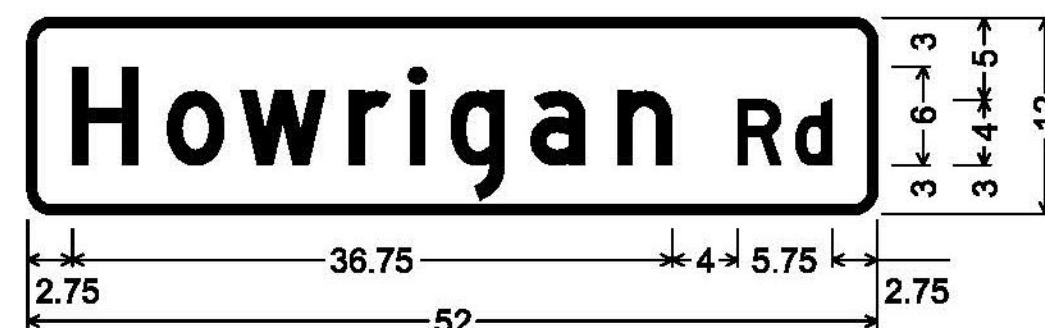
DOUBLE-SIDED STREET SIGN (ENOSBURGH); 1.500" Radius, 0.500" Border, White on Green; [Howrigan] D; [Rd] D;
