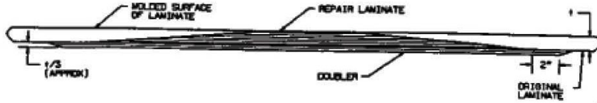
DOUBLER WITH SCARF ON NON-MOLDED SURFACE
