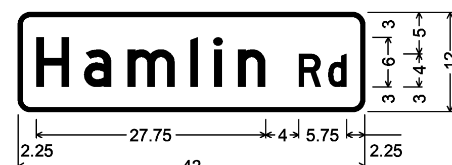
DOUBLE-SIDED STREET SIGN (CORNWALL); 1,500" Radius, 0.500" Border, White on Green; [Hamlin] D; [Rd] D;
