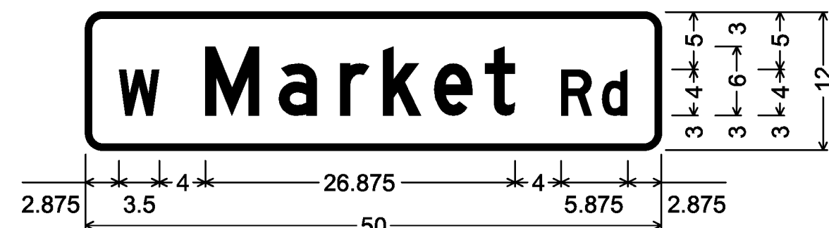
DOUBLE-SIDED STREET SIGN (BRIDPORT); 1,500" Radius, 0.500" Border, White on Green; [W] D; [Market] D; [Rd] D;
