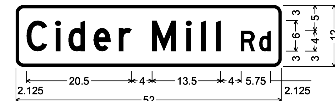
DOUBLE-SIDED STREET SIGN (CORNWALL); 1,500" Radius, 0.500" Border, White on Green; [Cider Mill] D; [Rd] D;
