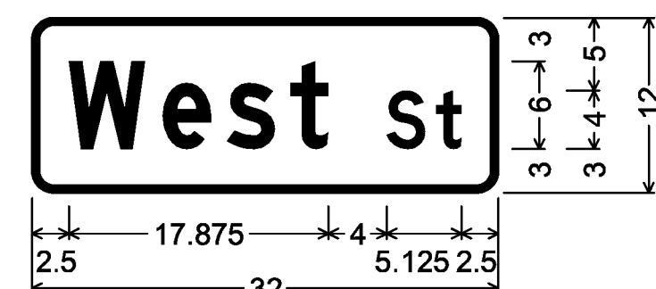
DOUBLE-SIDED STREET SIGN (CORNWALL); 1,500" Radius, 0.500" Border, White on Green; [West] D; [St] D;
