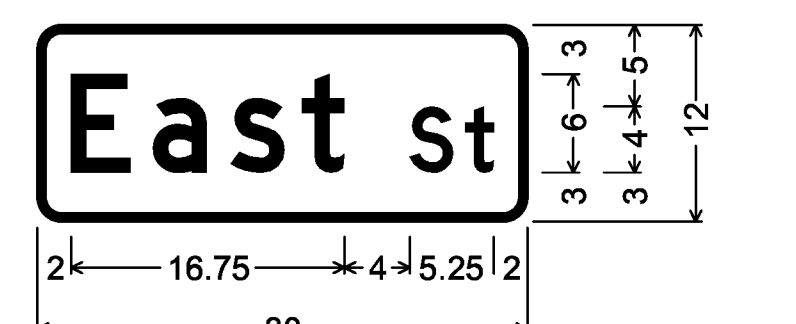
DOUBLE-SIDED STREET SIGN (BRIDPORT); 1,500" Radius, 0.500" Border, White on Green; [East] D; [St] D;
