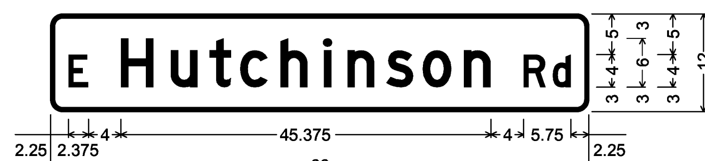
DOUBLE-SIDED STREET SIGN (BRIDPORT); 1.500" Radius, 0.500" Border, White on Green; [E] D; [Hutchinson] D; [Rd] D;
