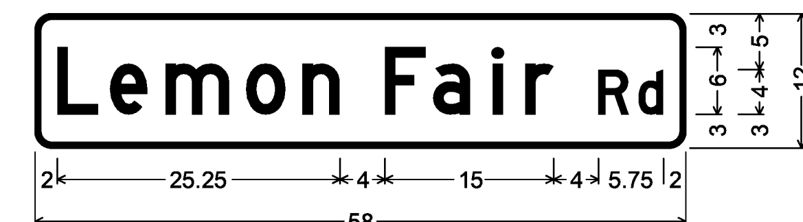
DOUBLE-SIDED STREET SIGN (CORNWALL); 1.500" Radius, 0.500" Border, White on Green; [Lemon Fair] D; [Rd] D;
