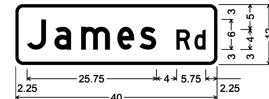
DOUBLE-SIDED STREET SIGN (CORNWALL); 1.500" Radius, 0.500" Border, White on Green; [James] D; [Rd] D;
