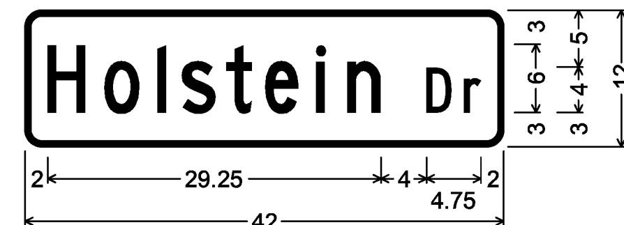
DOUBLE-SIDED STREET SIGN (BRIDPORT); 1.500" Radius, 0.500" Border, White on Green; [Holstein] C; [Dr] C;
