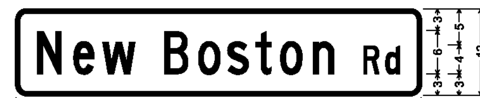
DOUBLE-SIDED STREET SIGN (POULTNEY); 1.500" Radius, 0.500" Border, White on Green; [New Boston] C; [Rd] C;
