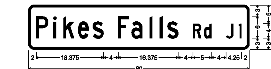
DOUBLE-SIDED STREET SIGN (JAMAICA); 1.500" Radius, 0.500" Border, White on Green; [Pikes Falls] C; [Rd] C; [J1] C;
