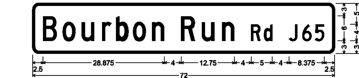
DOUBLE-SIDED STREET SIGN (JAMAICA); 1.500" Radius, 0.500" Border, White on Green; [Bourbon Run] C; [Rd] C; [J65] C;
