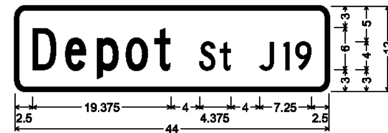
DOUBLE-SIDED STREET SIGN (JAMAICA); 1.500" Radius, 0.500" Border, White on Green; [Depot] C; [St] C; [J19] C;
