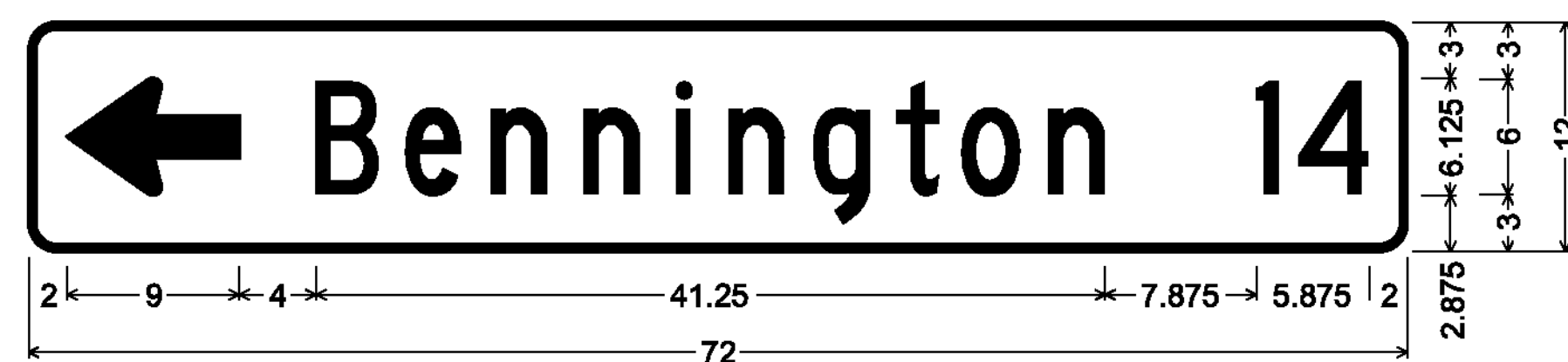
1.500" Radius, 0.375" Border, White on Green; Standard Arrow Custom 9.000" X 6.125" 180°; [Bennington] C; [14] C;
