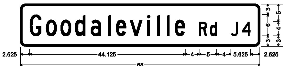
DOUBLE-SIDED STREET SIGN (JAMAICA); 1.500" Radius, 0.500" Border, White on Green; [Goodaleville] C; [Rd] C; [J4] C;
