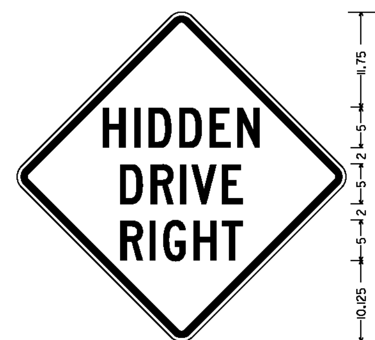
30.00" ACROSS SIDES, 1.875" RADIUS, 0.750" BORDER, 0.500" INDENT, BLACK ON YELLOW; [HIDDEN] 5", [DRIVE] 5", [RIGHT] 5"
