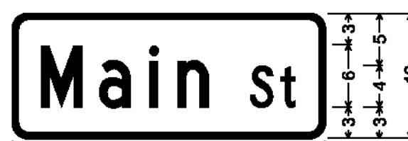
DOUBLE-SIDED STREET SIGN (POWNA); 1.500" Radius, 0.500" Border, White on Green; [Main] C; [St] C;
