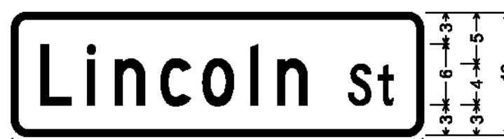
DOUBLE-SIDED STREET SIGN (POWNA); 1.500" Radius, 0.500" Border, White on Green; [Lincoln] C; [St] C;
