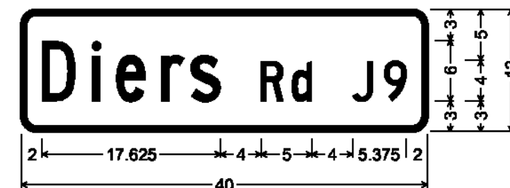
DOUBLE-SIDED STREET SIGN (JAMAICA); 1.500" Radius, 0.500" Border, White on Green; [Diers] C; [Rd] C; [J9] C;
