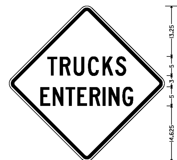
30.00" ACROSS SIDES, 1.875" RADIUS, 0.750" BORDER, 0.500" INDENT, BLACK ON YELLOW; [TRUCKS] 5", [ENTERING] 5" @ 80% SPACING
