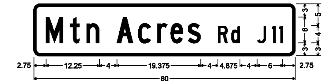
DOUBLE-SIDED STREET SIGN (JAMAICA); 1.500" Radius, 0.500" Border, White on Green; [Mtn Acres] C; [Rd] C; [J11] C;
