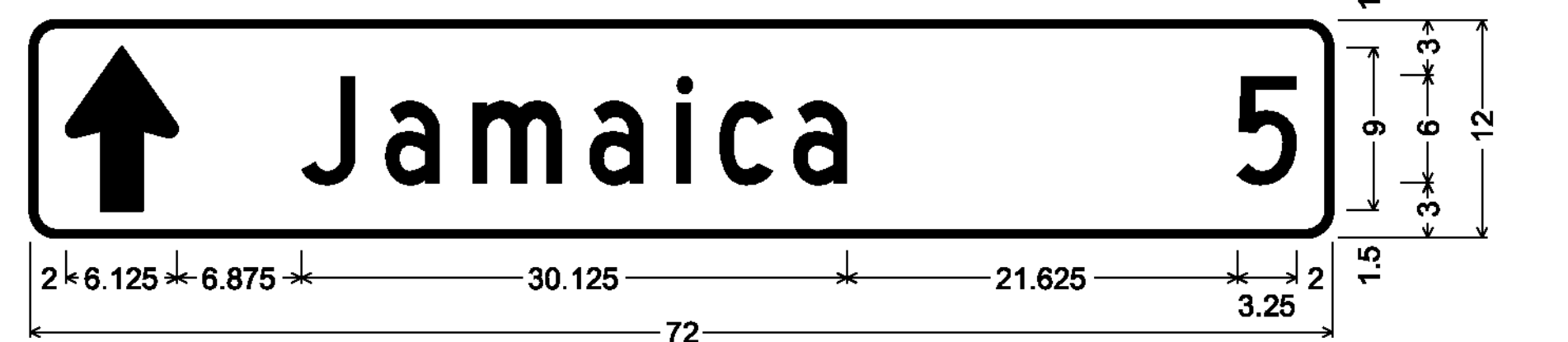
1.500" Radius, 0.375" Border, White on Green; Standard Arrow Custom 9.000" X 6.125" 90°; [Jamaica] C; [5] C;
