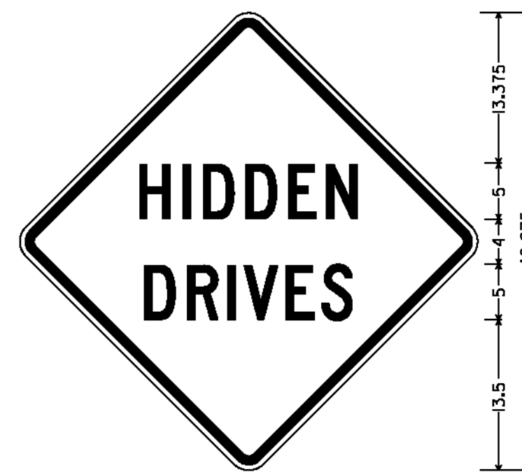
30.00" ACROSS SIDES, 1.875" RADIUS, 0.750" BORDER, 0.500" INDENT, BLACK ON YELLOW; [HIDDEN] 5", [DRIVES] 5"
