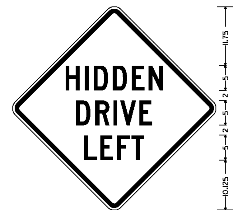
30.00" ACROSS SIDES, 1.875" RADIUS, 0.750" BORDER, 0.500" INDENT, BLACK ON YELLOW; [HIDDEN] 5", [DRIVE] 5", [LEFT] 5"
