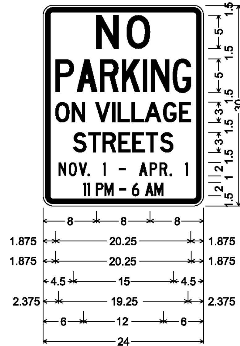
R8-1 MOD. 1.500" Radius, 0.625" Border, 0.375" Indent, Red on White; [NO] D; [PARKING] C specified length; [ON VILLAGE] D 50% spacing; [STREETS] D 50% spacing; [NOV. 1 - APR. 1] C specified length; [11 PM - 6 AM] C 45% spacing;
