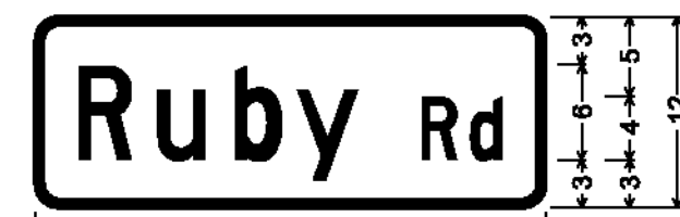
DOUBLE-SIDED STREET SIGN (POULTNEY); 1.500" Radius, 0.500" Border, White on Green; [Ruby] C; [Rd] C;
