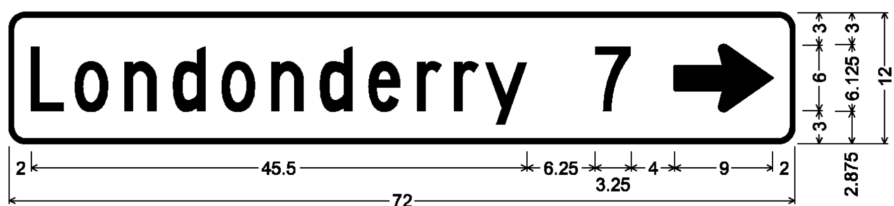
1.500" Radius, 0.375" Border, White on Green; [Londonderry] C; [7] C; Standard Arrow Custom 9.000" X 6.125" 0°;
