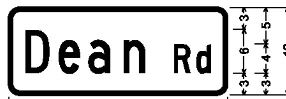
DOUBLE-SIDED STREET SIGN (POWNA); 1.500" Radius, 0.500" Border, White on Green; [Dean] C; [Rd] C;
