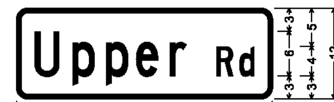
DOUBLE-SIDED STREET SIGN (POULTNEY); 1.500" Radius, 0.500" Border, White on Green; [Upper] C; [Rd] C;
