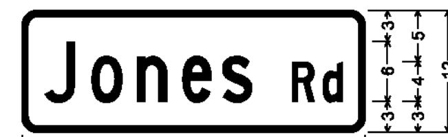
DOUBLE-SIDED STREET SIGN (POULTNEY); 1.500" Radius, 0.500" Border, White on Green; [Jones] C; [Rd] C;
