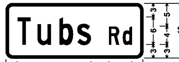
DOUBLE-SIDED STREET SIGN (POWNA); 1.500" Radius, 0.500" Border, White on Green; [Tubs] C; [Rd] C;
