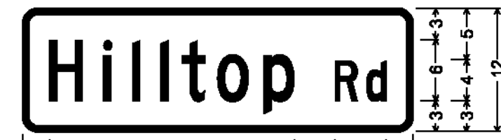
DOUBLE-SIDED STREET SIGN (WELLS); 1.500" Radius, 0.500" Border, White on Green; [Hilltop] C; [Rd] C;
