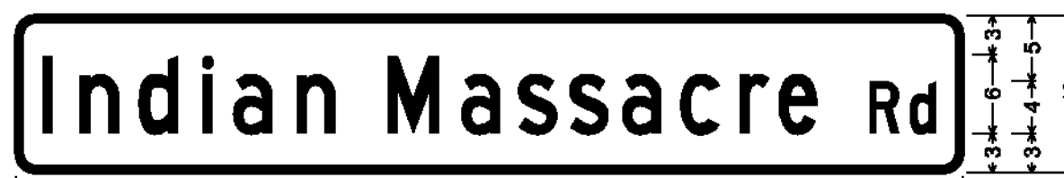
DOUBLE-SIDED STREET SIGN (POWNA); 1.500" Radius, 0.500" Border, White on Green; [Indian Massacre] C; [Rd] C;
