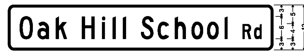
DOUBLE-SIDED STREET SIGN (POWNA); 1.500" Radius, 0.500" Border, White on Green; [Oak Hill School] C; [Rd] C;
