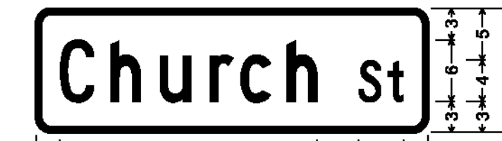
DOUBLE-SIDED STREET SIGN (POWNA); 1.500" Radius, 0.500" Border, White on Green; [Church] C; [St] C;
