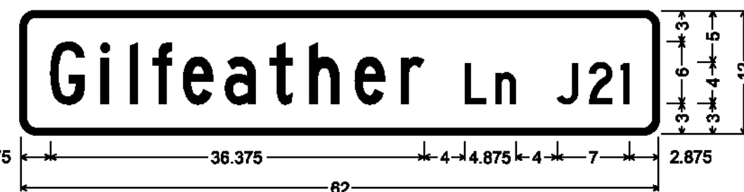
DOUBLE-SIDED STREET SIGN (JAMAICA); 1.500" Radius, 0.500" Border, White on Green; [Gilfeather] C; [Ln] C; [J21] C;
