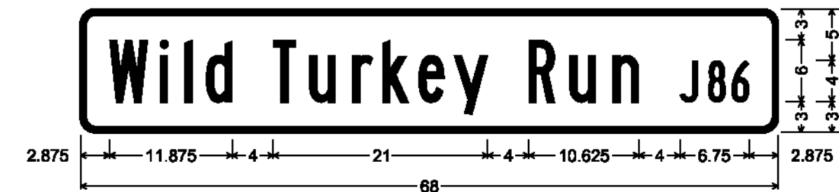
DOUBLE-SIDED STREET SIGN (JAMAICA); 1.500" Radius, 0.500" Border, White on Green; [Wild Turkey Run] B || C; [J86] B;
