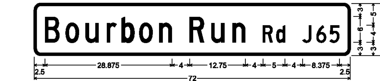
DOUBLE-SIDED STREET SIGN (JAMAICA); 1.500" Radius, 0.500" Border, White on Green; [Bourbon Run] C; [Rd] C; [J65] C;
