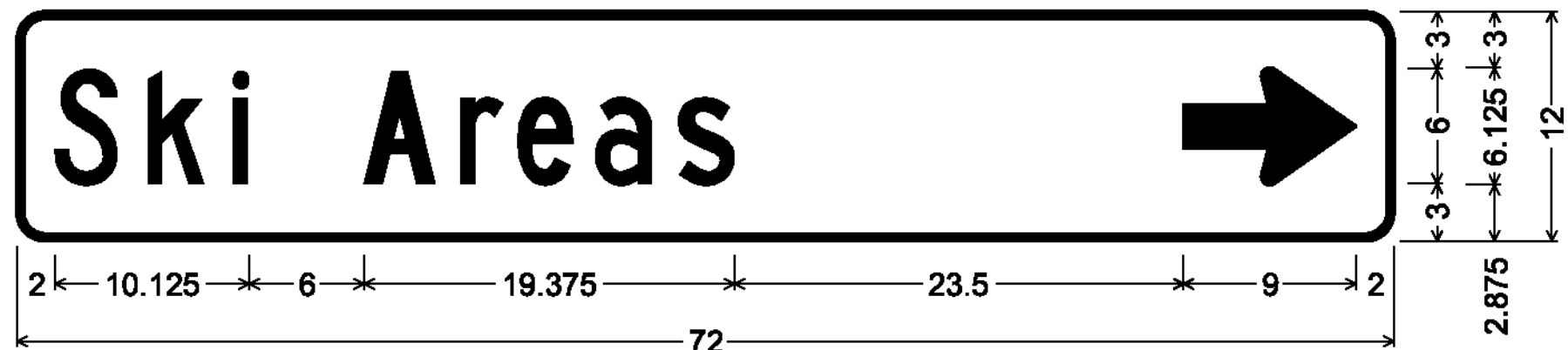
1.500" Radius, 0.375" Border, White on Green; [Ski Areas] C; Standard Arrow Custom 9.000" X 6.125" 0°;
