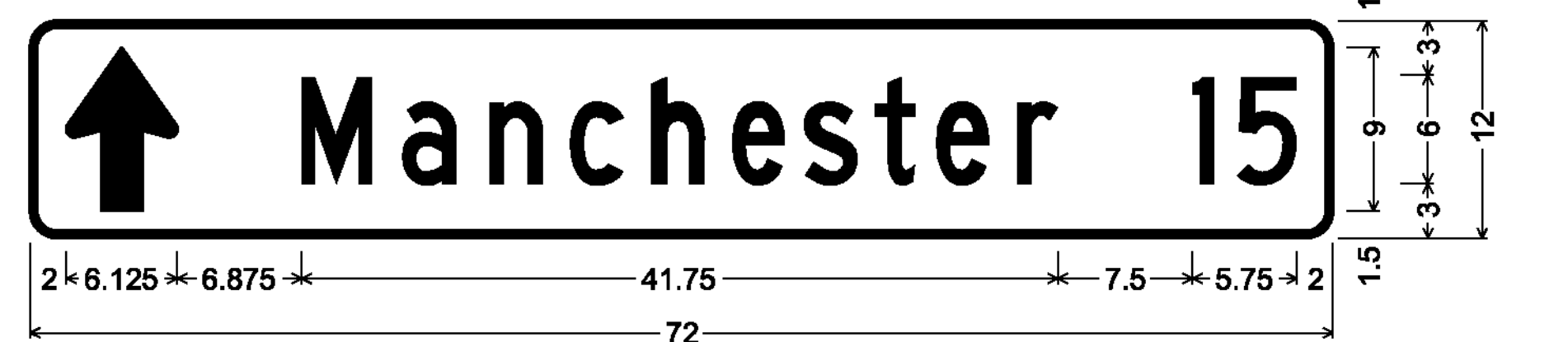
1.500" Radius, 0.375" Border, White on Green; Standard Arrow Custom 9.000" X 6.125" 90°; [Manchester] C; [15] C;
