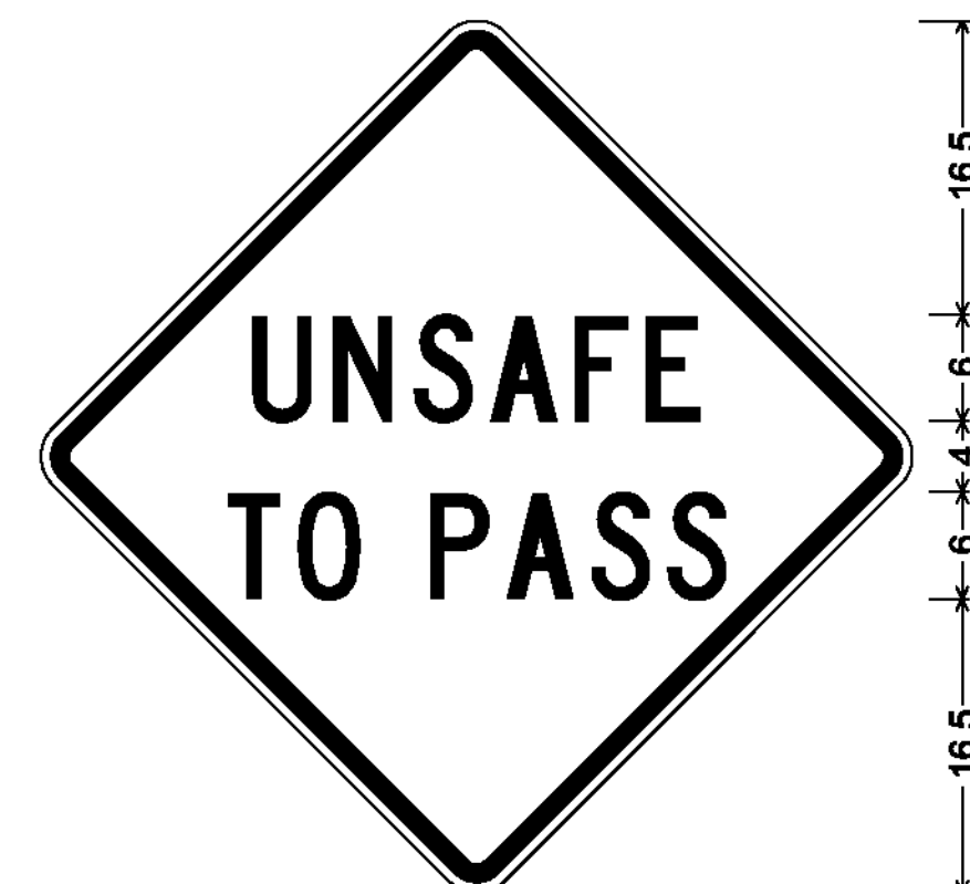
36.000" across sides 2.250" Radius, 0.875" Border, 0.625" Indent, Black on Yellow; [UNSAFE] C; [TO PASS] C;
