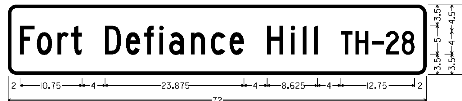
1,500" RADIUS, 0,500" BORDER, WHITE ON GREEN; [Fort Defiance Hill] 5"C, [TH-28] 4"C @ 80% SPACING
