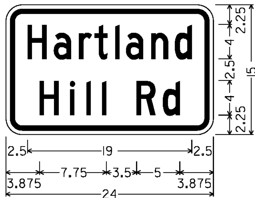
1,875" RADIUS, 0.500" BORDER, 0.500" INDENT, BLACK ON YELLOW; [Hartland] 4"C, [Hill] 4"C, [Rd] 4"C W16-8aP
