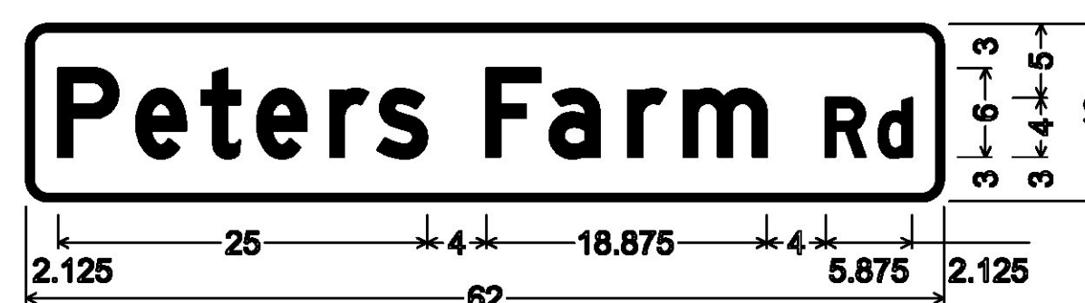
DOUBLE-SIDED STREET SIGN (SOUTH HERO); 1.500" Radius, 0.500" Border, White on Green; "Peters Farm" D; "Rd" D;
