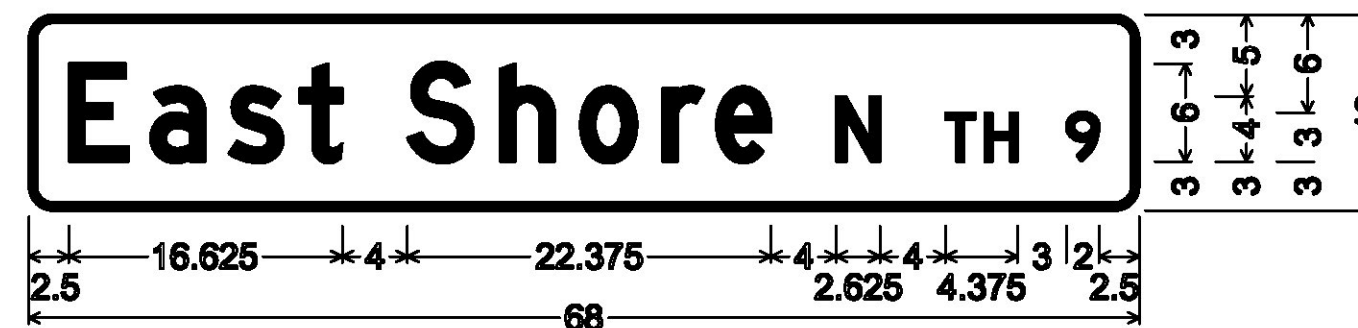
DOUBLE-SIDED STREET SIGN (GRAND ISLE); 1.500" Radius, 0.500" Border, White on Green; "East Shore" D; "N" D; "TH 9" D;
