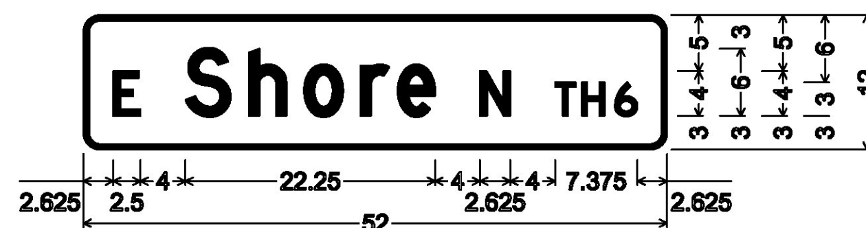
DOUBLE-SIDED STREET SIGN (GRAND ISLE); 1.500" Radius, 0.500" Border, White on Green; "E" D; "Shore" D; "N" D; "TH6" D;
