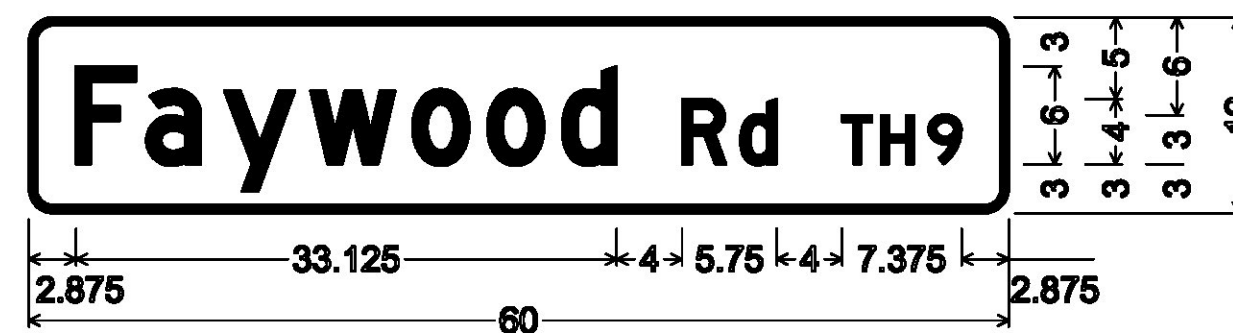
DOUBLE-SIDED STREET SIGN (GRAND ISLE); 1.500" Radius, 0.500" Border, White on Green; "Faywood" D; "Rd" D; "TH9" D;
