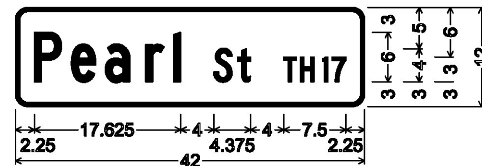
DOUBLE-SIDED STREET SIGN (GRAND ISLE); 1.500" Radius, 0.500" Border, White on Green; "Pearl" C; "St" C; "TH17" C;
