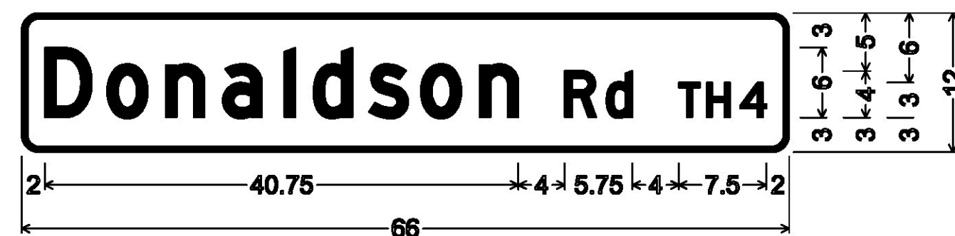
DOUBLE-SIDED STREET SIGN (GRAND ISLE); 1.500" Radius, 0.500" Border, White on Green; "Donaldson" D; "Rd" D; "TH4" D;
