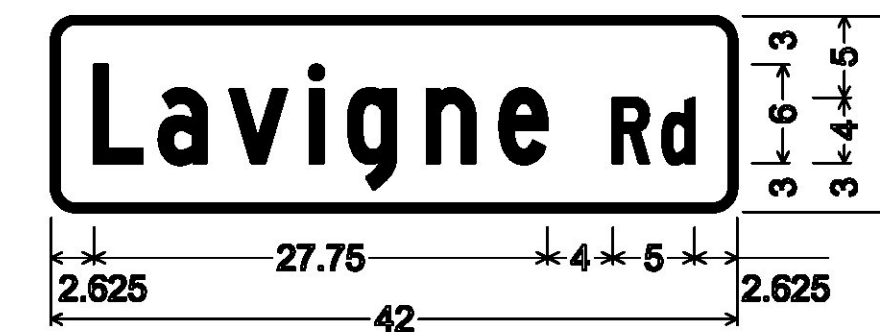
DOUBLE-SIDED STREET SIGN (SOUTH HERO); 1.500" Radius, 0.500" Border, White on Green; "Lavigne" C; "Rd" C;
