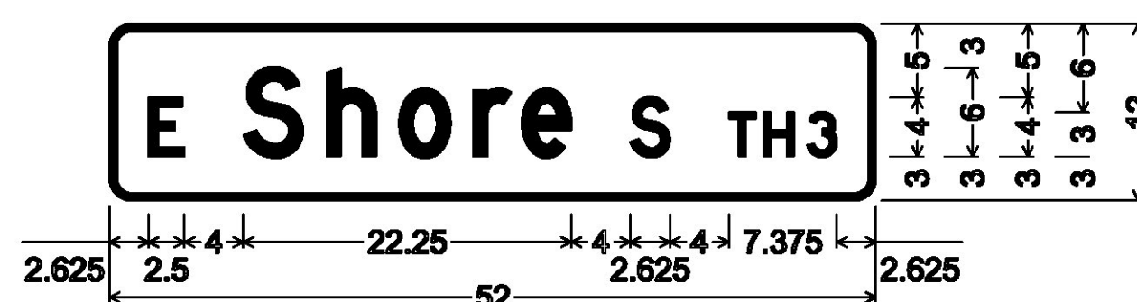
DOUBLE-SIDED STREET SIGN (GRAND ISLE); 1.500" Radius, 0.500" Border, White on Green; "E" D; "Shore" D; "S" D; "TH3" D;
