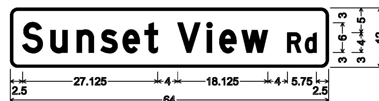
DOUBLE-SIDED STREET SIGN (NORTH HERO); 1.500" Radius, 0.500" Border, White on Green; "Sunset View" D; "Rd" D;
