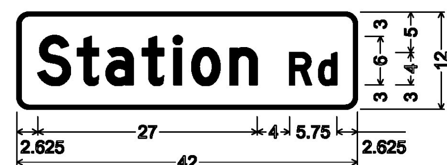
DOUBLE-SIDED STREET SIGN (NORTH HERO); 1.500" Radius, 0.500" Border, White on Green; "Station" D 80% spacing; "Rd" D;
