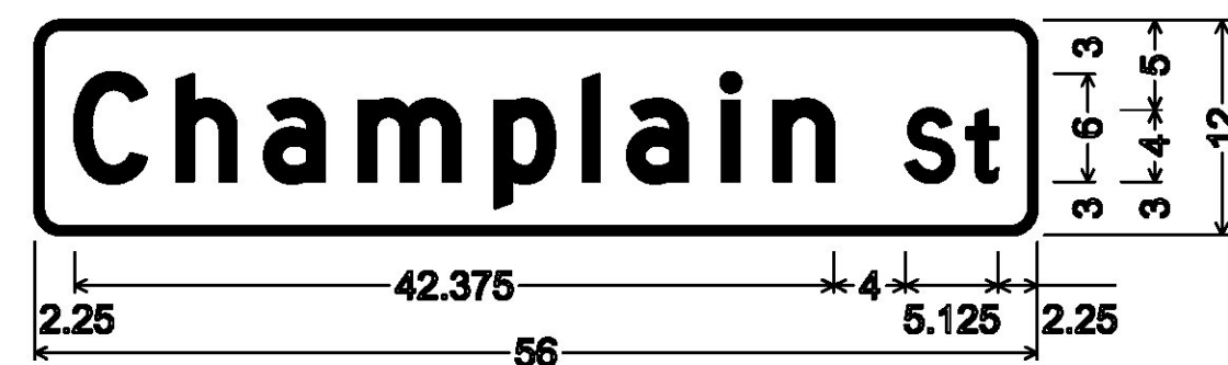
DOUBLE-SIDED STREET SIGN (ALBURGH); 1.500" Radius, 0.500" Border, White on Green; "Champlain" D; "St" D;
