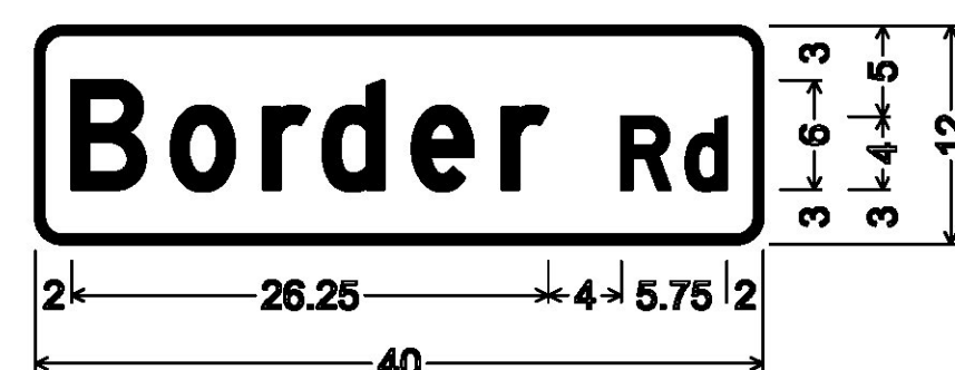
DOUBLE-SIDED STREET SIGN (ALBURGH); 1.500" Radius, 0.500" Border, White on Green; "Border" D; "Rd" D;
