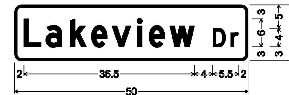
DOUBLE-SIDED STREET SIGN (NORTH HERO); 1.500" Radius, 0.500" Border, White on Green; "Lakeview" D; "Dr" D;
