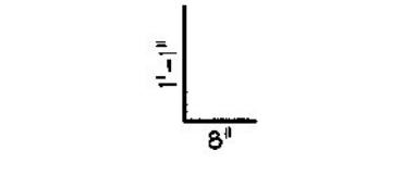
AN-505E #5 BENT BAR LEVEL I (EPOXY COATED) USE 2 3/4" Ø (70 mm) PIN (72) REQ'D.
