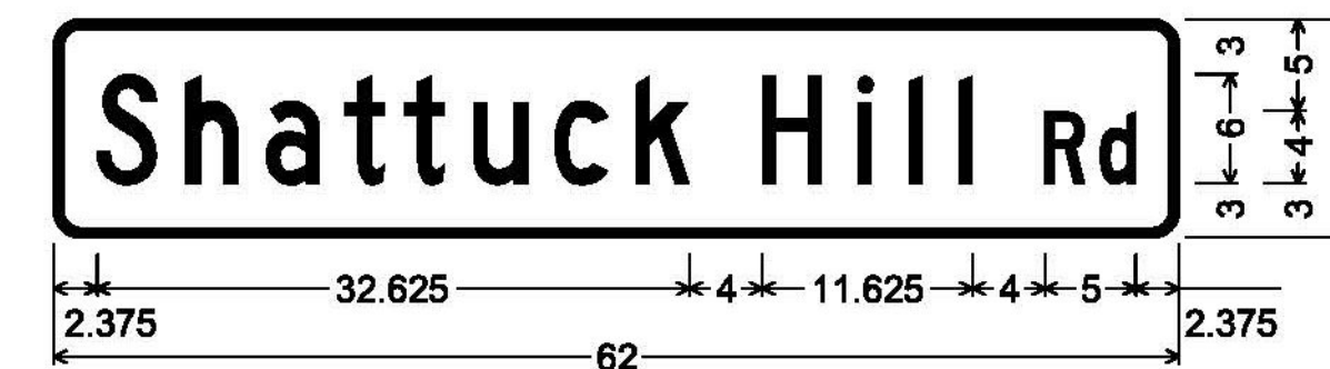
DOUBLE-SIDED STREET SIGN (DERBY); 1.500" Radius, 0.500" Border, White on Green; [Shattuck Hill] C; [Rd] C;
