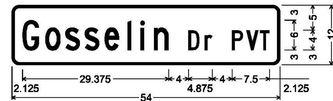
DOUBLE-SIDED STREET SIGN (DERBY); 1.500" Radius, 0.500" Border, White on Green; [Gosselin] C; [Dr PVT] C;
