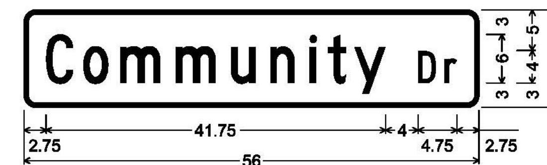
DOUBLE-SIDED STREET SIGN (DERBY); 1.500" Radius, 0.500" Border, White on Green; [Community] C; [Dr] C;
