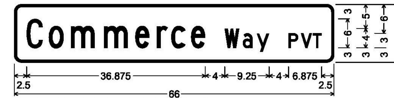
DOUBLE-SIDED STREET SIGN (DERBY); 1.500" Radius, 0.500" Border, White on Green; [Commerce] C; [Way] C; [PVT] D;
