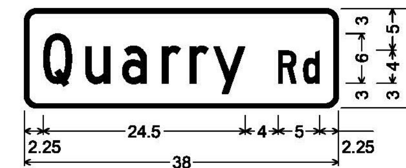
DOUBLE-SIDED STREET SIGN (DERBY); 1.500" Radius, 0.500" Border, White on Green; [Quarry] C; [Rd] C;
