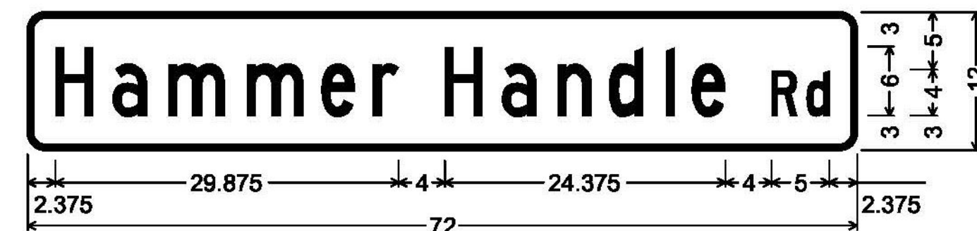
DOUBLE-SIDED STREET SIGN (DERBY); 1.500" Radius, 0.500" Border, White on Green; [Hammer Handle] C; [Rd] C;
