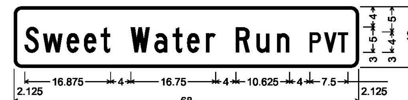
DOUBLE-SIDED STREET SIGN (DERBY); 1.500" Radius, 0.500" Border, White on Green; [Sweet Water Run] C; [PVT] C;
