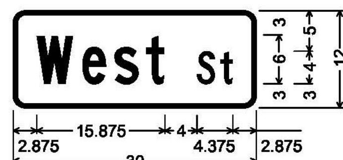
DOUBLE-SIDED STREET SIGN (DERBY); 1.500" Radius, 0.500" Border, White on Green; [West] C; [St] C;
