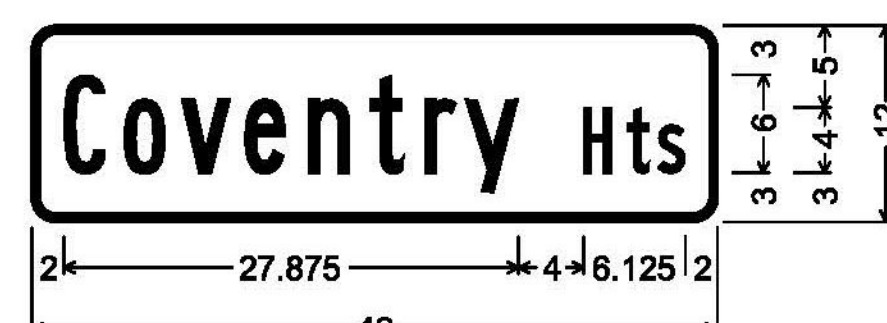
DOUBLE-SIDED STREET SIGN (COVENTRY); 1.500" Radius, 0.500" Border, White on Green; [Coventry] B; [Hts] B;
