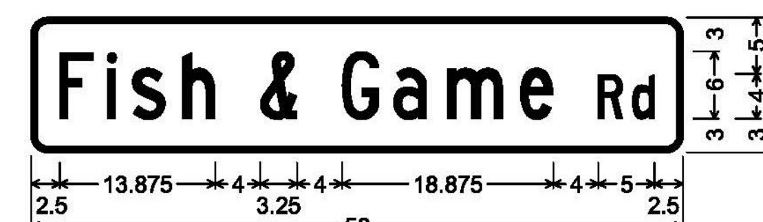
DOUBLE-SIDED STREET SIGN (DERBY); 1.500" Radius, 0.500" Border, White on Green; [Fish & Game] C; [Rd] C;
