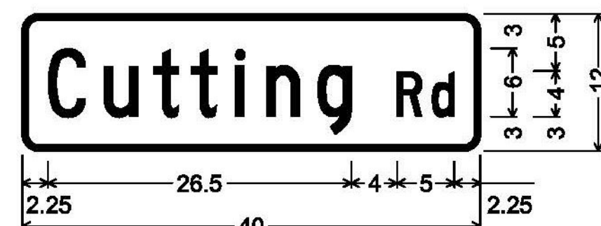
DOUBLE-SIDED STREET SIGN (IRASBURG); 1.500" Radius, 0.500" Border, White on Green; [Cutting] C; [Rd] C;
