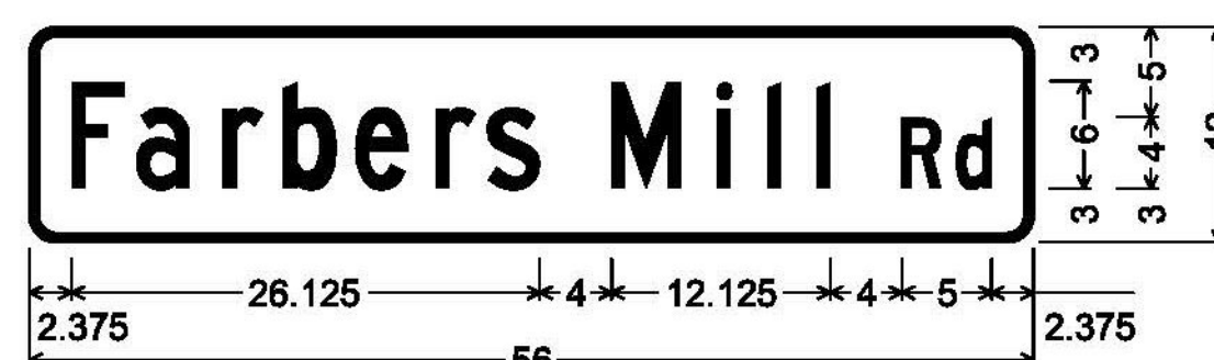
DOUBLE-SIDED STREET SIGN (COVENTRY); 1.500" Radius, 0.500" Border, White on Green; [Farbers Mill] C; [Rd] C;
