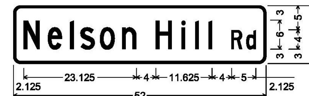
DOUBLE-SIDED STREET SIGN (DERBY); 1.500" Radius, 0.500" Border, White on Green; [Nelson Hill] C; [Rd] C;
