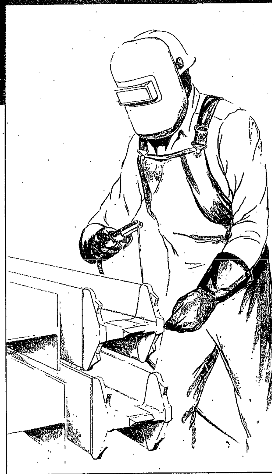
PROPERLY LOCATED SINGLE BEVEL GROOVE WELDS
