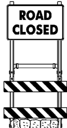
SIGN MOUNTING ON TYPE III BARRICADE (MODIFIED) (A)
