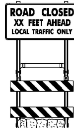
SIGN MOUNTING ON TYPE III BARRICADE (MODIFIED) (B)
