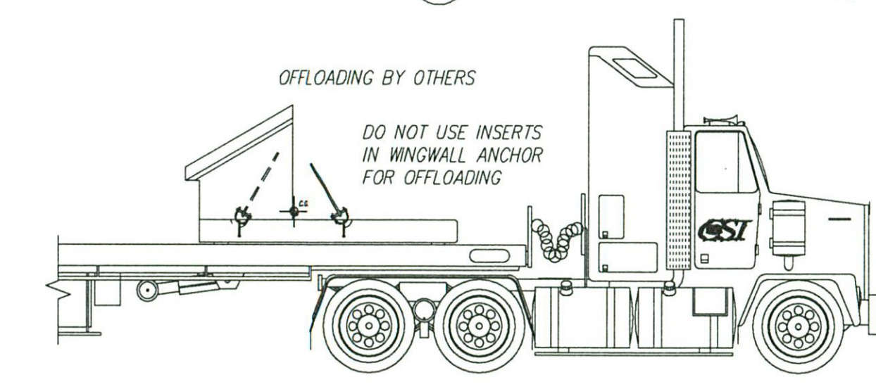
S TYPICAL WINGWALL OFFLOADING DETAIL Scale: N.T.S.
