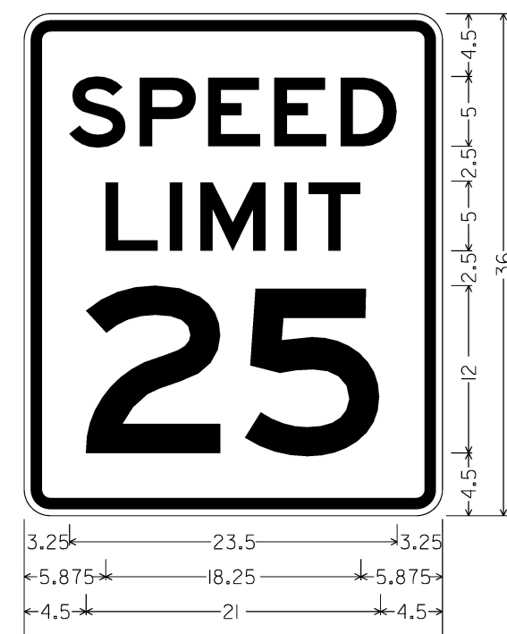
1/8" RADIUS, 0.750" BORDER, 0.500" INDENT, BLACK ON WHITE; [SPEED] 5"E; [LIMIT] 5"E; [25] 12"E
