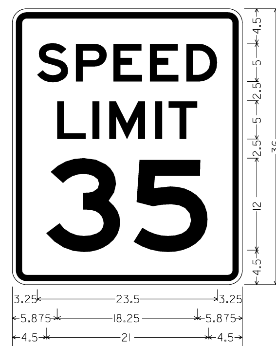
1/8" RADIUS, 0.750" BORDER, 0.500" INDENT, BLACK ON WHITE; [SPEED] 5"E; [LIMIT] 5"E; [35] 12"E
