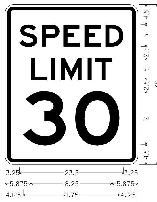
1/8" RADIUS, 0.750" BORDER, 0.500" INDENT, BLACK ON WHITE; [SPEED] 5"E; [LIMIT] 5"E; [30] 12"E
