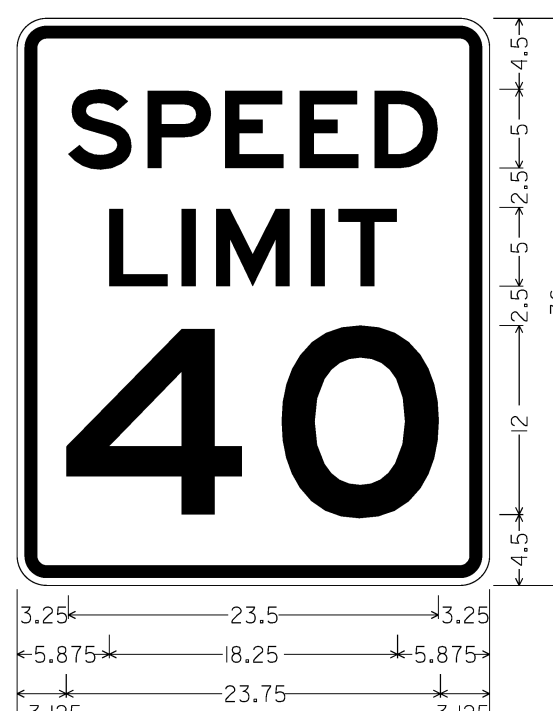
1/8" RADIUS, 0.750" BORDER, 0.500" INDENT, BLACK ON WHITE; [SPEED] 5"E; [LIMIT] 5"E; [40] 12"E
