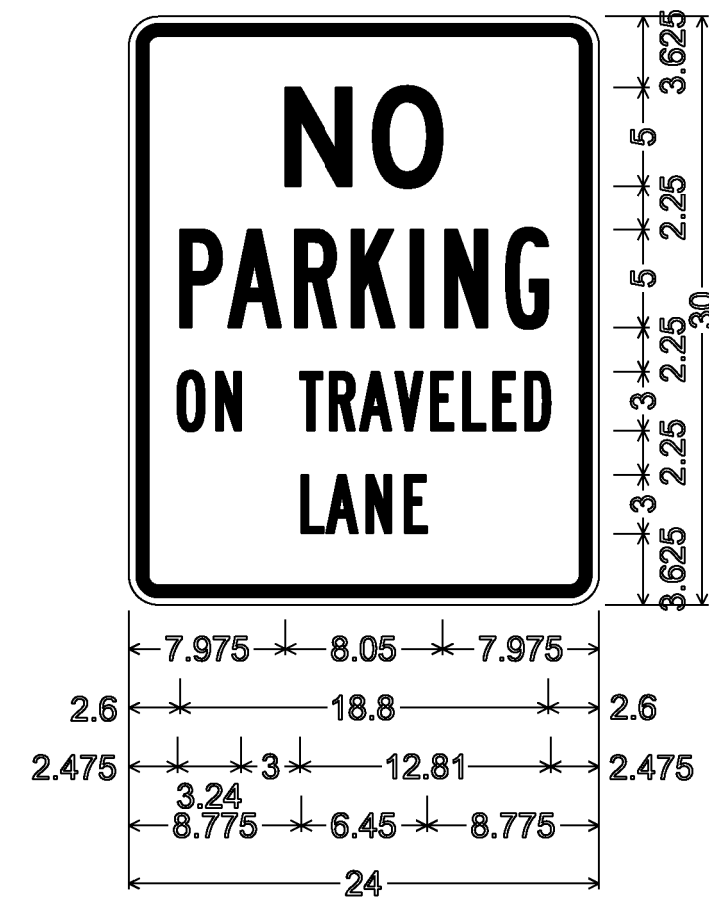
VR-020; 1.500" Radius, 0.625" Border, 0.375" Indent, Red on White; "NO" D 2K; "PARKING" B 2K; "ON TRAVELED" B 2K; "LANE" B 2K;
