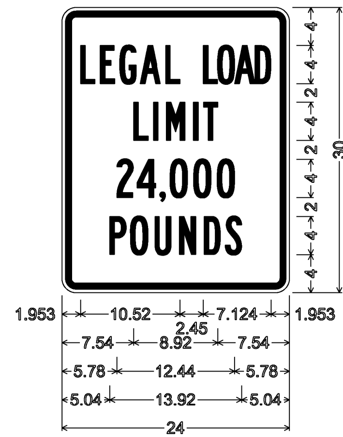
VR-017; 1.500" Radius, 0.625" Border, 0.375" Indent, Black on White; "LEGAL" B 2K "LOAD" Highway B; "LIMIT" B 2K; "24,000" B 2K; "POUNDS" B 2K;
