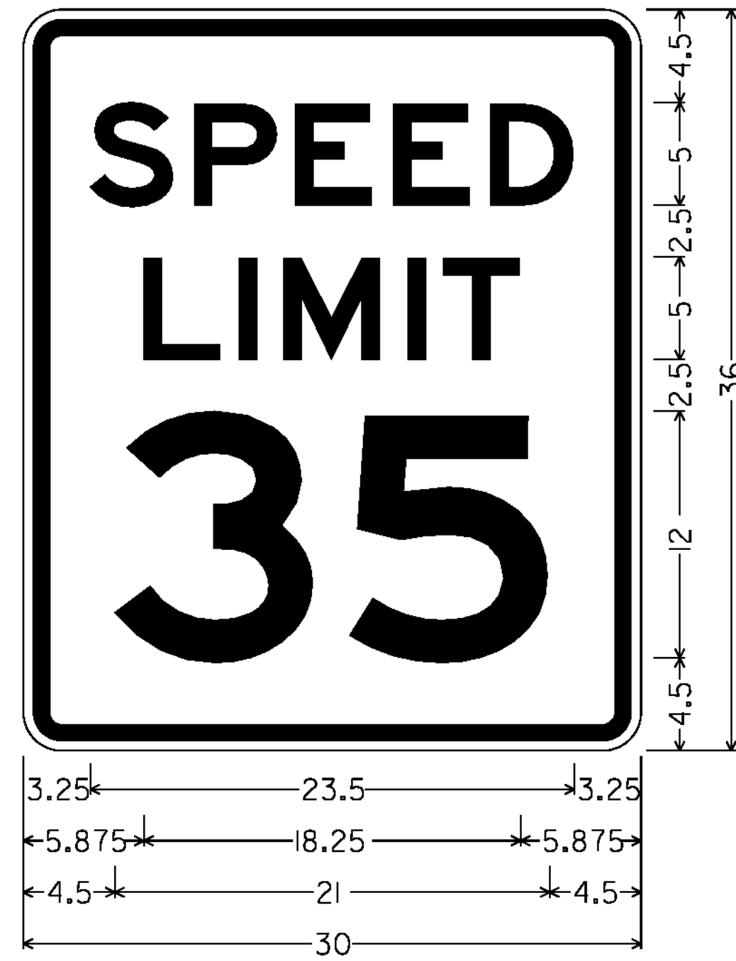
1.875" RADIUS, 0.750" BORDER, 0.500" INDENT, BLACK ON WHITE; [SPEED] 5"E; [LIMIT] 5"E; [35] 12"E R2-1
