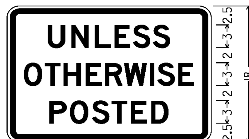
1.500" RADIUS, 0.625" BORDER, 0.375" INDENT, BLACK ON WHITE; [UNLESS] 2"D; [OTHERWISE] 2"D; [POSTED] 2"D R2-5P
