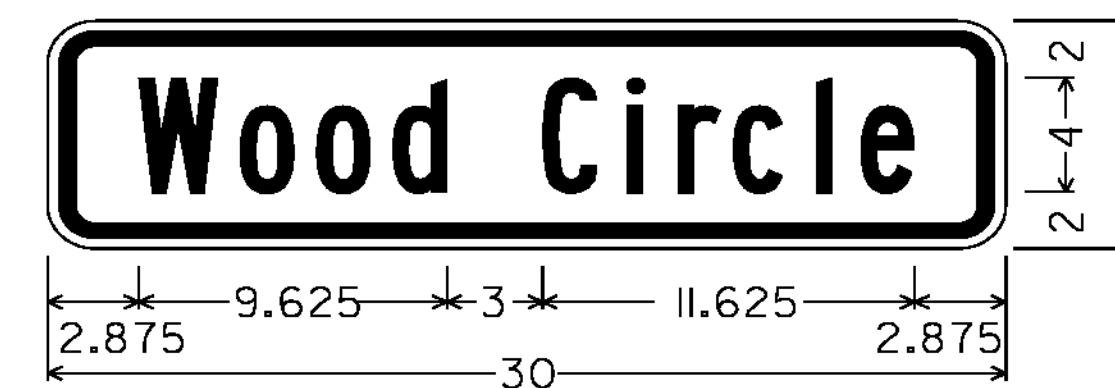
1.500" RADIUS, 0.500" BORDER, 0.375" INDENT, BLACK ON YELLOW; [Wood Circle] 4"B W16-8P
