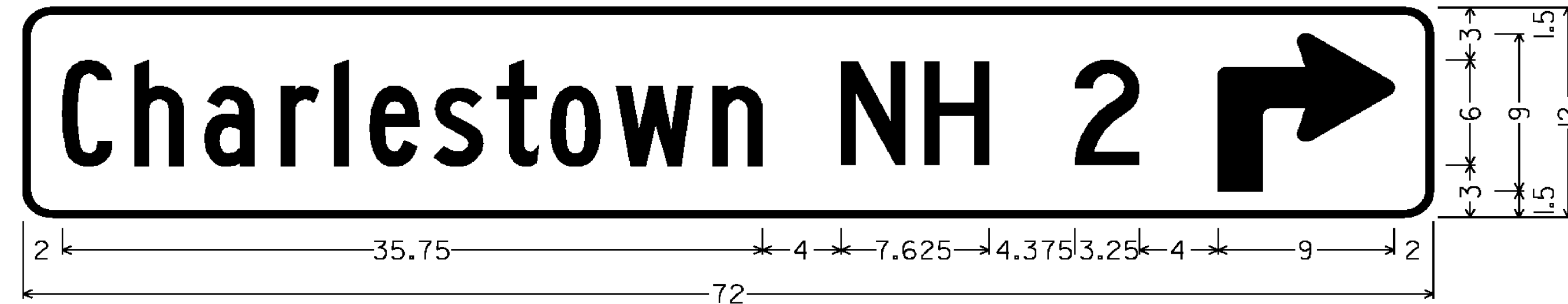
1.500" RADIUS, 0.375" BORDER, WHITE ON GREEN; [Charlestown] 6"B; [NH] 6"C; [2] 6"C; 90 DEG ADVANCE TURN ARROW 9.000" X 9.000" VDI-IA
