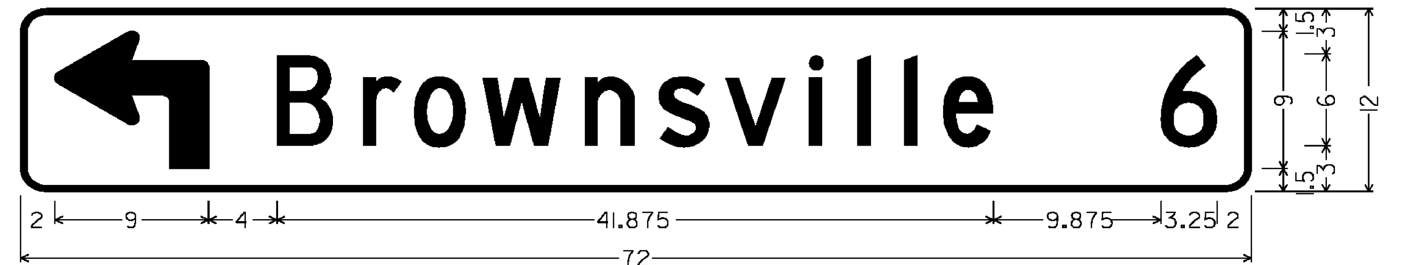
1.500" RADIUS, 0.375" BORDER, WHITE ON GREEN; 90 DEG ADVANCE TURN ARROW 9.000" X 9.000"; [Brownsville] 6"C; [6] 6"C VDI-IA
