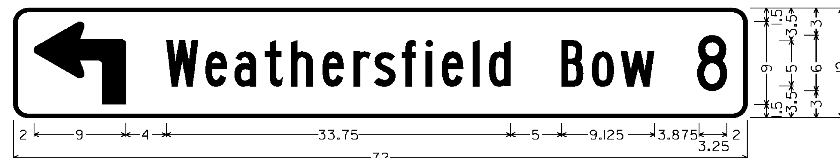
1.500" RADIUS, 0.375" BORDER, WHITE ON GREEN; 90 DEG ADVANCE TURN ARROW 9.000" X 9.000"; [Weathersfield Bow] 5"B; [8] 6"C VDI-IA
