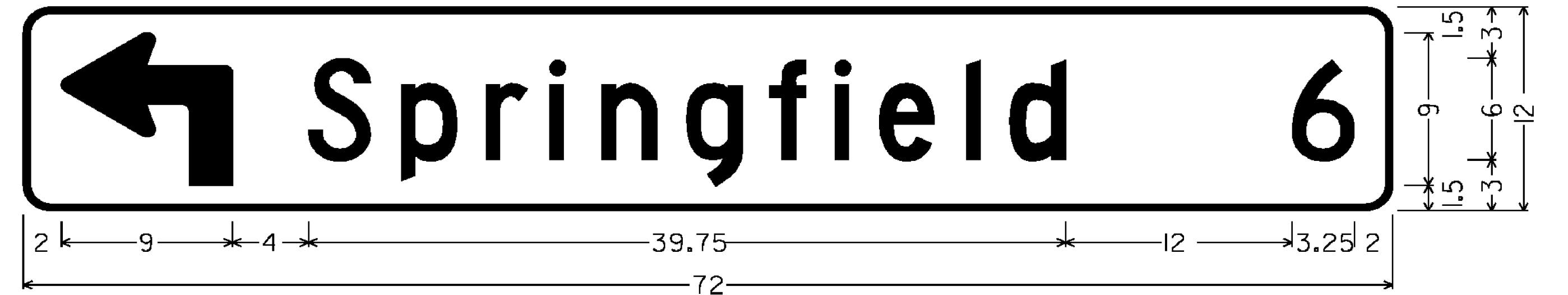
1.500" RADIUS, 0.375" BORDER, WHITE ON GREEN; 90 DEG ADVANCE TURN ARROW 9.000" X 9.000"; [Springfield] 6"C; [6] 6"C VDI-IA
