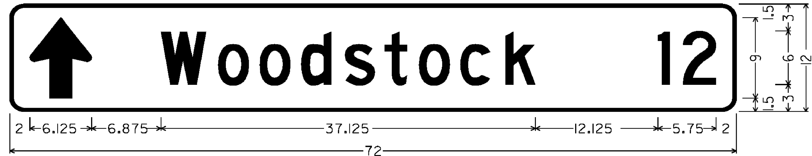
1.500" RADIUS, 0.375" BORDER, WHITE ON GREEN; STANDARD ARROW 9.000" X 6.125" @ 90 DEG; [Woodstock] 6"C; [12] 6"C VDI-IA
