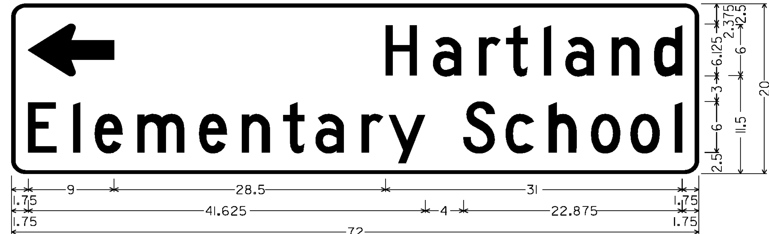
1.500" RADIUS, 0.375" BORDER, WHITE ON GREEN; STANDARD ARROW 9.000" X 6.125" @ 180 DEGREES; [Hartland] 6"C; [Elementary] 6"C; [School] 6"C VDI-2L
